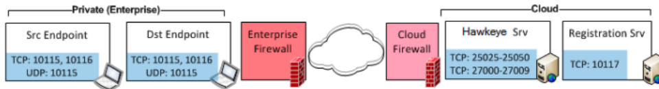
Figure 3.12: Test scenario with source and destination endpoint in same Enterprise network, and HS and RS in the Cloud [17].
