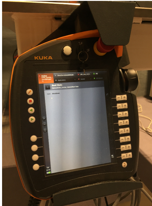
Figure 3.11.: Teach pendant from KUKA.
