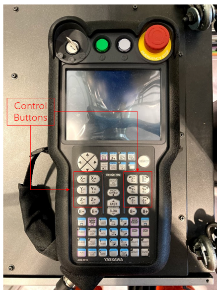
Figure 7.4.: The teach pendant connected to the YRC1000 robot controller. Control buttons for each joint are marked by the red squares.
