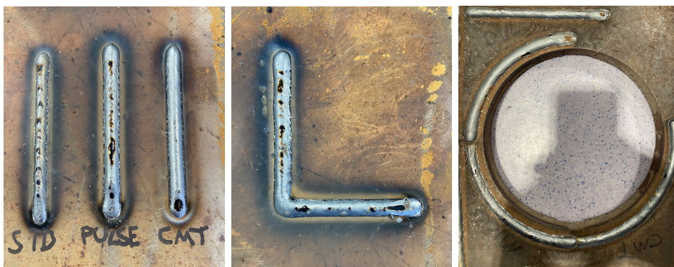
Figure 9.1.: Welding seams from the three different welding operations. Left: straight welds with three different welding methods: MIG, MIG pulse and CMT. Middle: welding an angle. Right: welding a circle using the positioning table.
