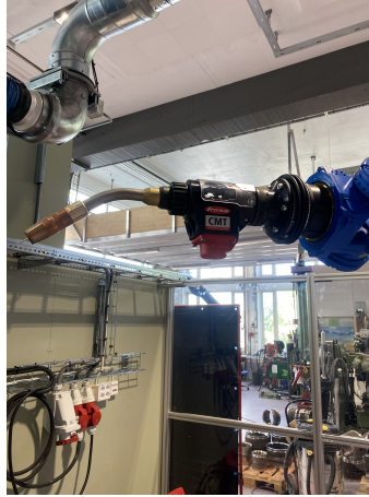
Figure 4.4.: Close-up of wrist and the attached welding gun
