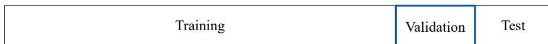
Figure 2.13: An illustration of how the data should be divided into a training set, validation set and test set.
