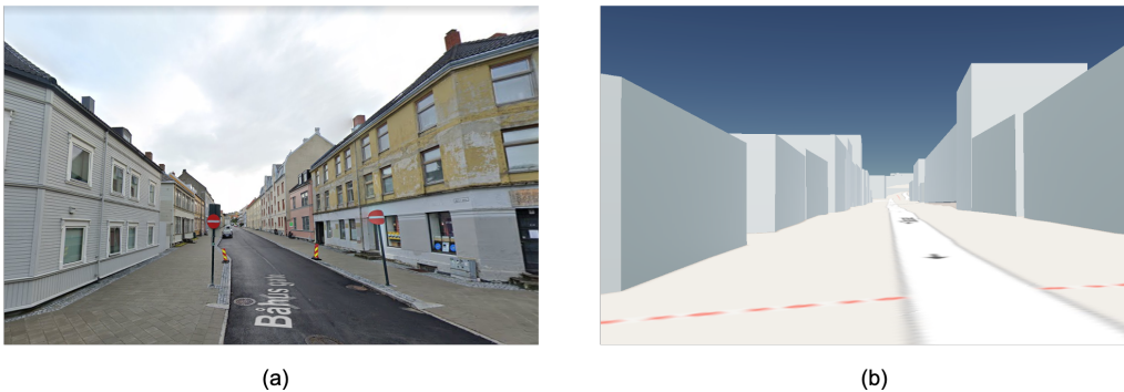
Figure 21: This figure shows a comparison between a street view image with a shop floor (a) and its corresponding, one-story, 3D model representation (b). ((a): Google, "Streetview," digital images, Google Maps (GoogleMaps 2021), photograph of Båhus gate, 7030, Trondheim, captured: Aug 2020)
