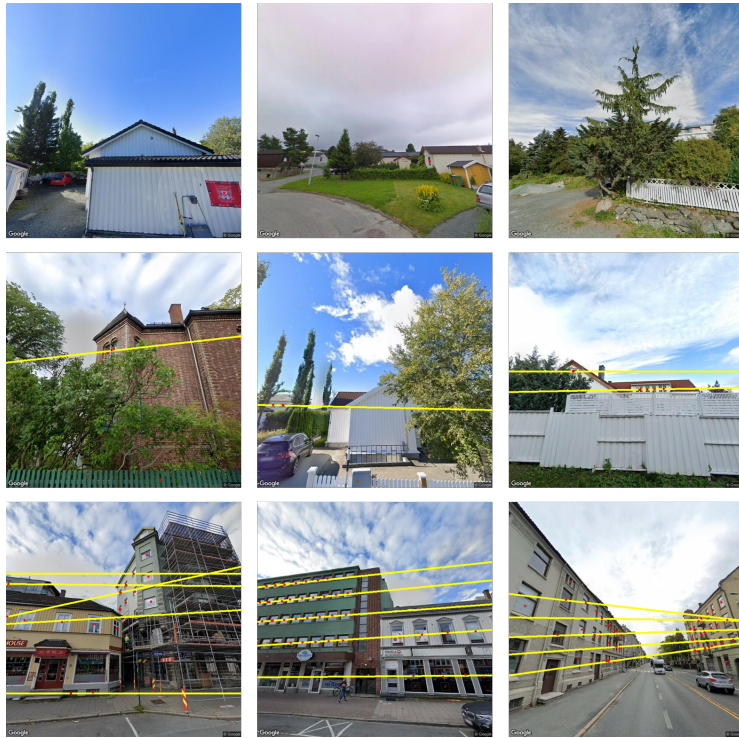
Figure 15: Example visualization of the floor segmentation results on street-level imagery that was either incorrectly positioned, occluded, misaligned, or included background noise.
