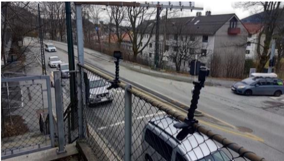
Figure 5.2: Mounting of cameras at intersection 1
