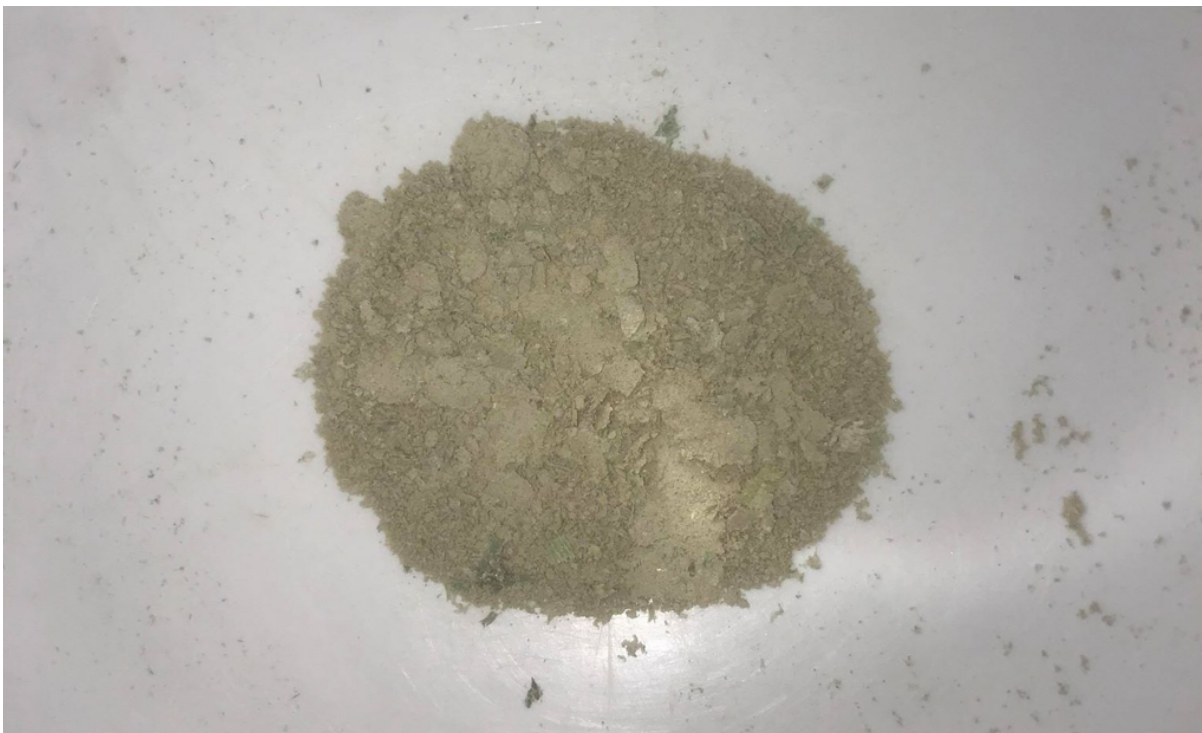
Picture 4: Homogenized powder of dry matter content of all polychaetes from the same replicate (tank) in the feeding trial. Visible fragments likely to be chitin from exoskeleton. Photo: Bjørn Kristensen
