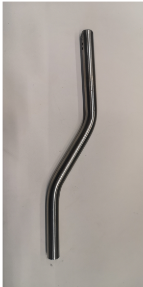
(a) The new CO 2 insertion pipe
