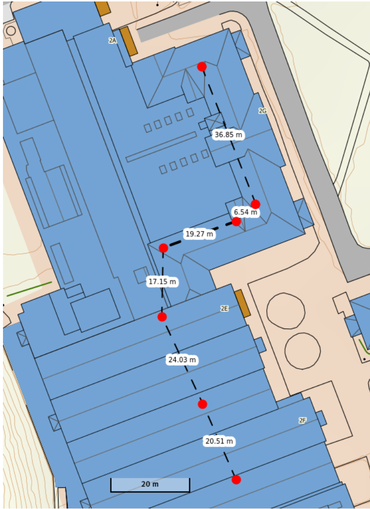
Figure 47: Map from revised node placement. The distance marked 6.54m is larger in reality, due to altitude.
