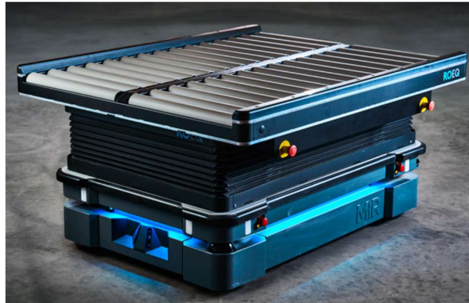
Figure 5.6 – Special top module AMR (Conveyor top), collected from Mobile Industrial Robots A/S (2021f)
