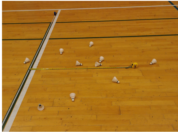
Figure 38: Placement of the shuttles from the second tube with slightly used shuttles
