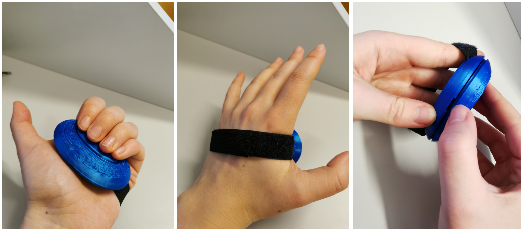
Figure 69: The first prototype attached to a hand and using the notch to open it
