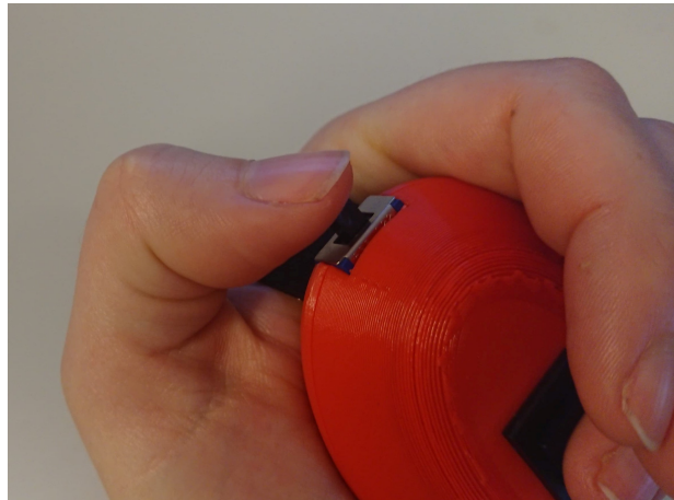
Figure 82: A button on top of the case can in future development be used to e.g. switch between different modes
