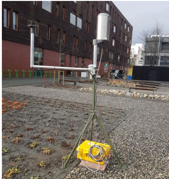
Figure 8: Weather station installed at the ZEB-laboratory site
