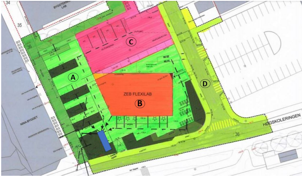
Figure 4: Overview of areas connected to the stormwater tank at the ZEB-building with piping roughly illustrated. Area A: Permeable surface and bioretention cells; Area B: ZEB-lab roof; Area C: Parking lot; Area D: Existing road. Stormwater tank in blue, located in lower left corner. Adapted from Pedersen (2020).
