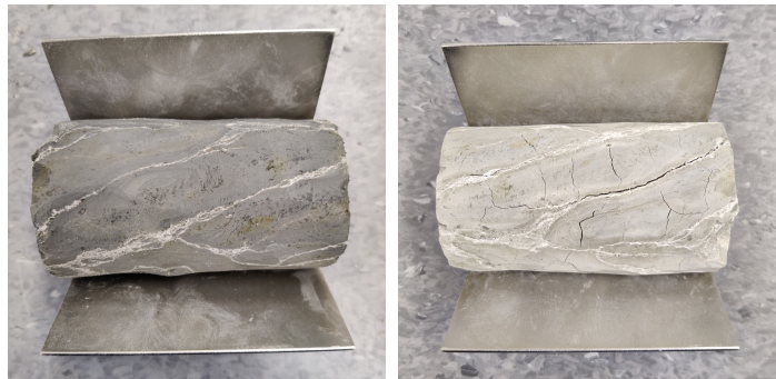
Figure 4.10: CT-scans sample drying. F15 before and after CT
