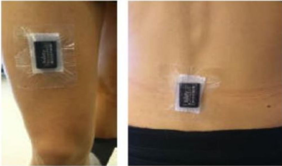
Figure 2.1: The placement of the accelerometer sensors. The first image shows a sensor placed on a person's thigh. The second image shows sensor placement on the lower back.
