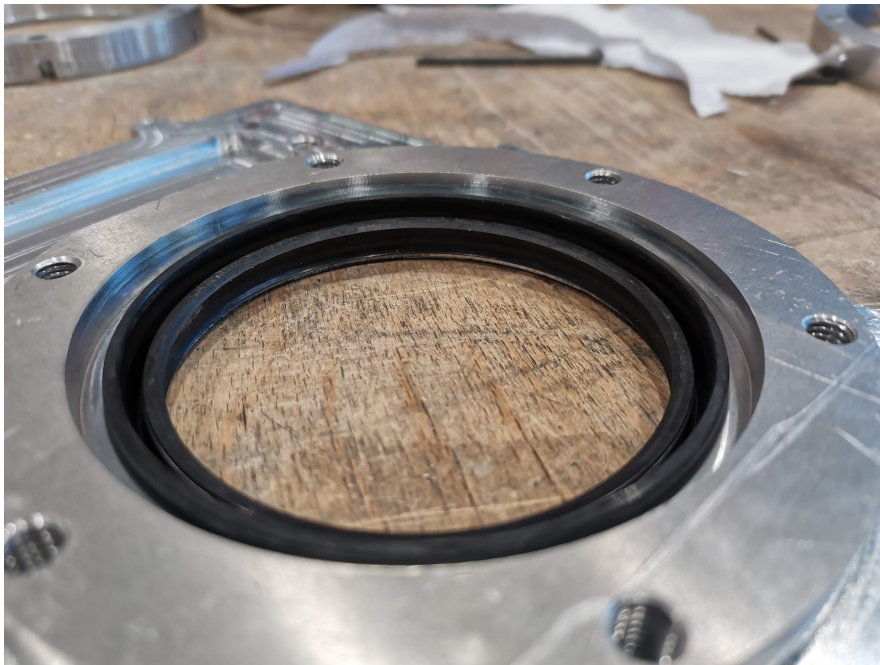
Figure 4.15: The sealing ring fitted into the bottom plate.
