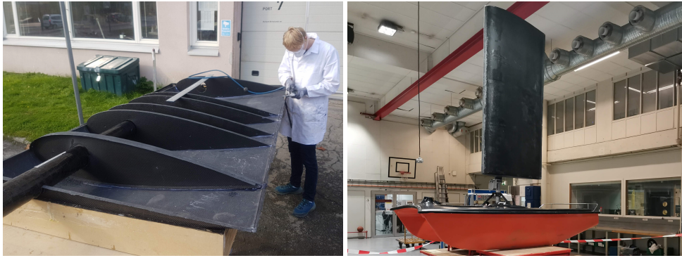
Figure 3.1: (a) Assembly of the CFRP wing. Notice the specific placement of the internal structure. (b) CFRP wing atop catamaran test hull.
