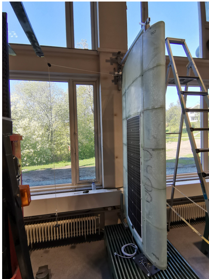
Figure 5.1: Full experimental setup for wing stiffness and actuation testing.
