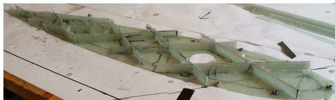
(a) Crossing reinforcement is added under the bottom wing section.
