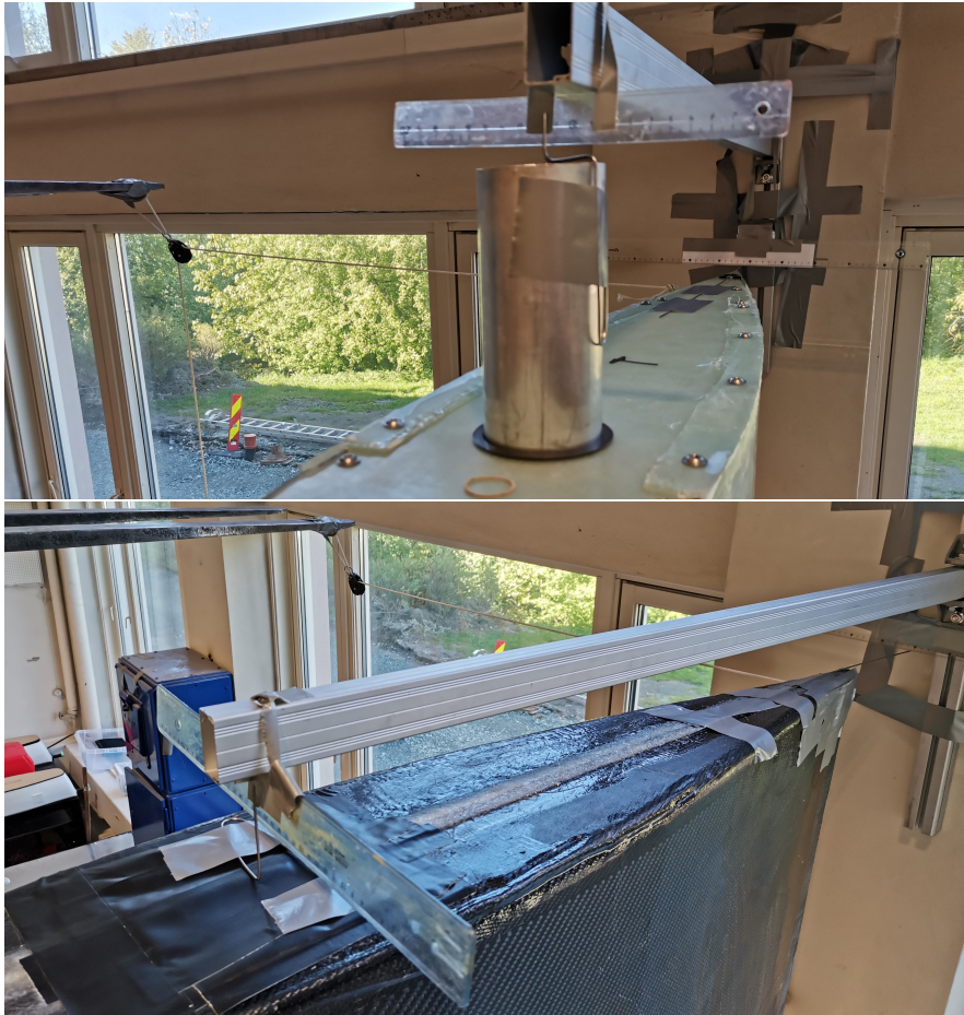
Figure 5.2: Experimental setup for both wings. One ruler above the mast axis and one behind the trailing edge. The line running to the pulley and down to the load can also be seen.
