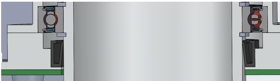
Figure 3.24: Sealing ring (black) sitting tight below the bearing in the bottom plate.
