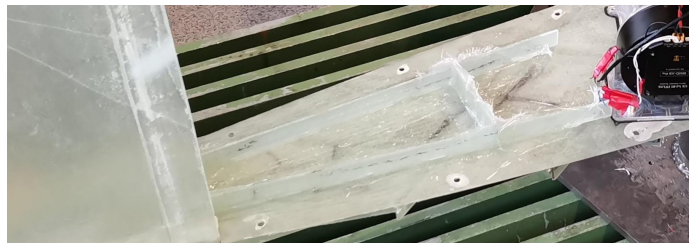
(b) The bottom section is reinforced in the longitudinal direction on the upside, to increase bending stiffness.
