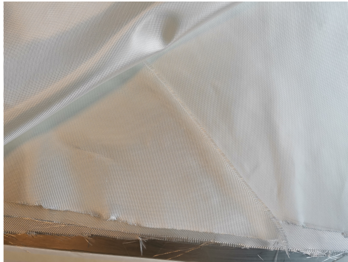
Figure 4.8: The overlapping joint in a ply oriented at 45^\circ .
