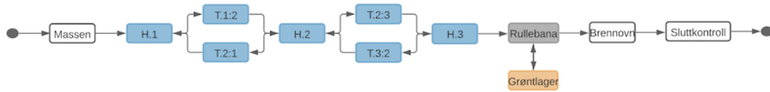
Figure 40: Overview of sub-system 1 - The overhead conveyor ( hengebana )
