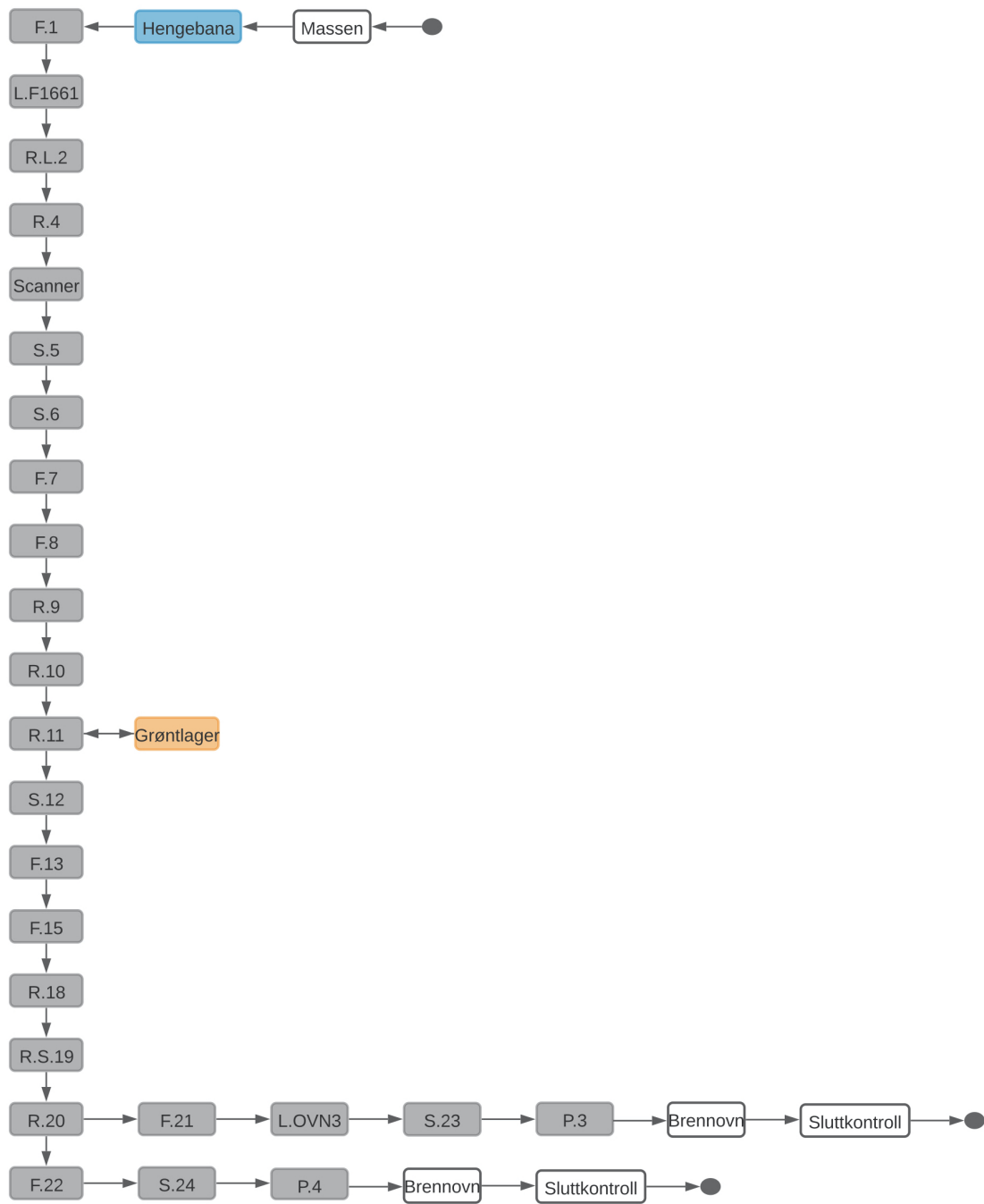
Figure 41: Overview of sub-system 2 - The roller conveyor ( rullebana )
