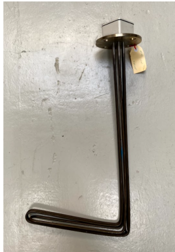
Figure 7: Picture of a heating element identical to the one used in the current system
