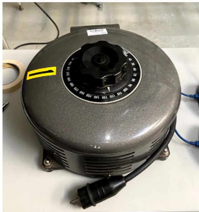
Figure 21: Picture of the controller to adjust the voltage
