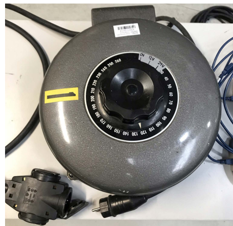
(b) The transformer used to change the voltage.
