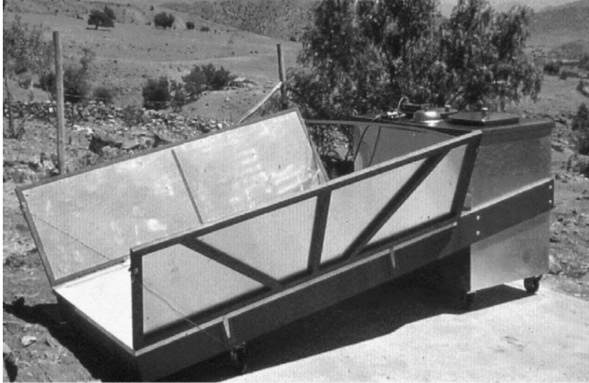
Figure 2.4: Flat-plate solar cooker with heat storage installed in an elementary school in Chile [32].
