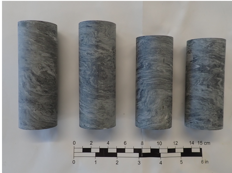
Figure 7.3: Photo of UCS-1, UCS-2, UCS-3 and UCS-4 (from left to right) before testing.
