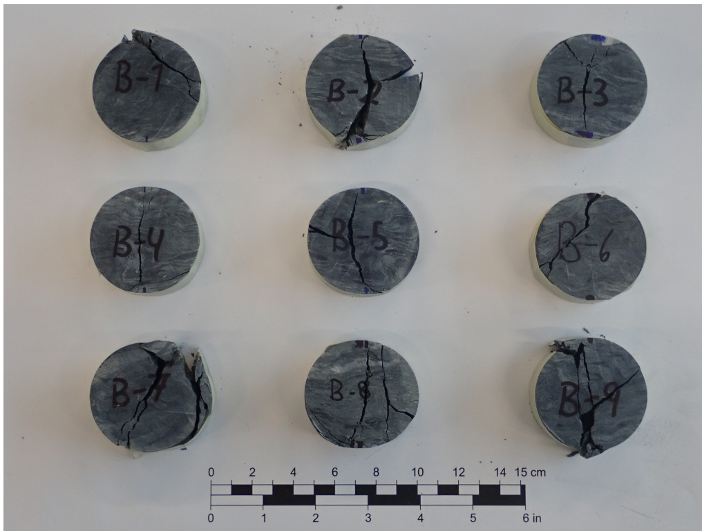
Figure 7.8: Photo of samples B-1 to B-9 after tensile failure. B-1 and B-6 have invalid failure.
