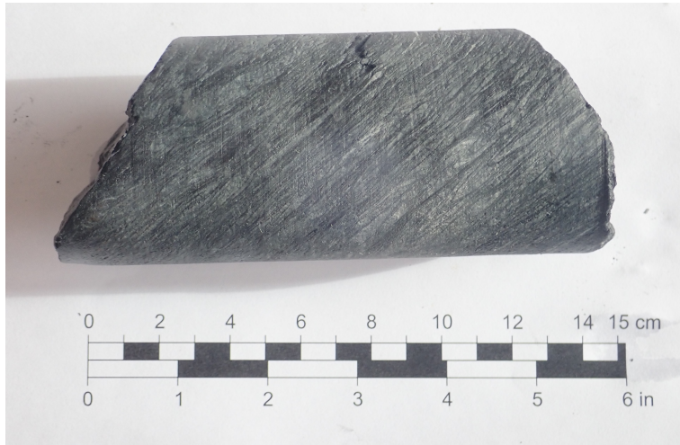
Figure 7.9: Picture of the specimen illustrating the direction of the foliation plane.
