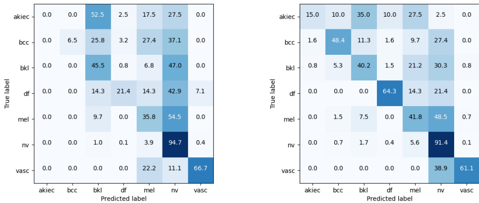
Figure 4.22: Confusion matrix UAP after both mitigation method, Inception V3 (Left) & Resnet 50 (Right)
