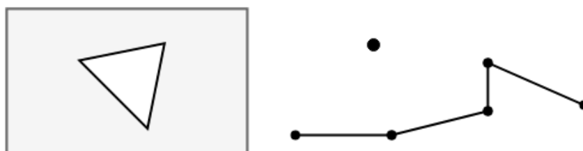
Figure 1: Geometries: Point, Linestring and Polygon (with an internal hole).
