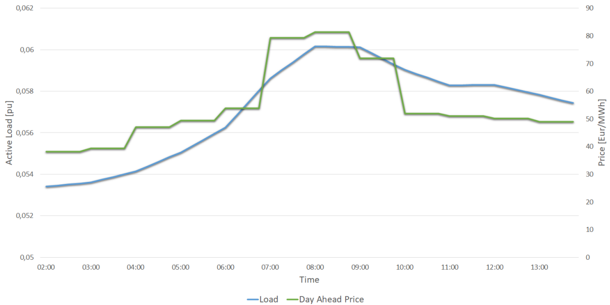
Figure 12: Correlation between the total load profile of the distribution grid and the day ahead prices.
