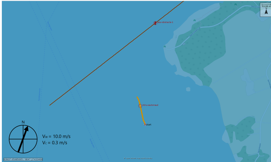
(a) Crossing from starboard scenario with static and dynamic obstacles and with environmental factors.
