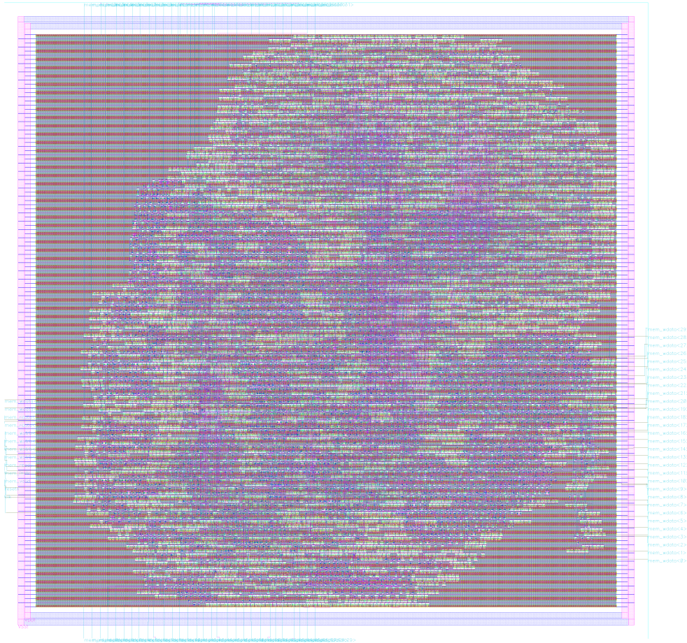
Fig. 10: Layout of PicoRV32 after P&R
