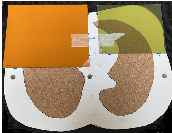
Figure 3.10: A transversal slice of the anthropomorphic female thorax phantom is shown. Here the GafChromic EBT3 film is positioned so that it covers the left breast, that is to be irradiated. The GafChromic XR-QA2 film is placed so that it covers the contralateral (opposite, here right) breast.
