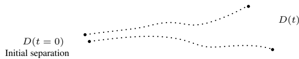
Figure 2.3: Qualitative sketch of the transport of a particle pair with separation D(t) .
