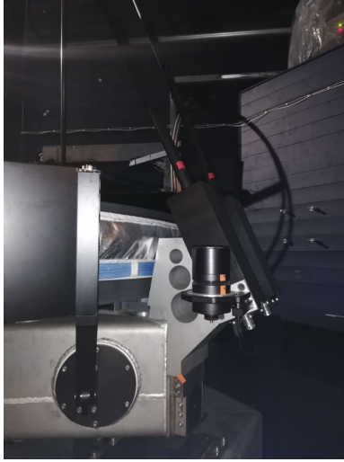
Figure A.1: The secondary telescope mounted to the side of the primary telescope.
