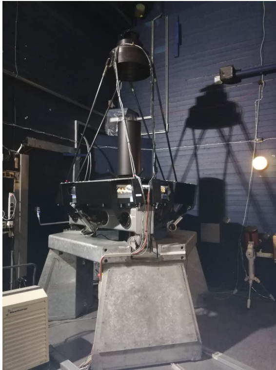
Figure 3.2: The cassegrain telescope for IAPs RMR-Lidar situated at ALOMAR.
