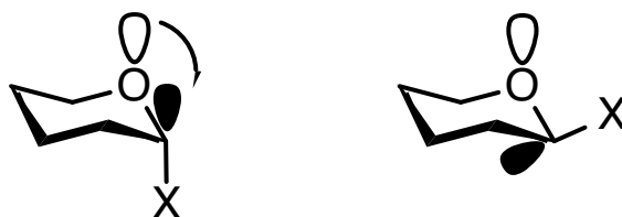
Figure 1.5. Model to explain anomeric effect by use of orbital interactions. 10,12 Black orbital indicates an antibonding orbital, while the white orbital indicates a nonbonding orbital.
