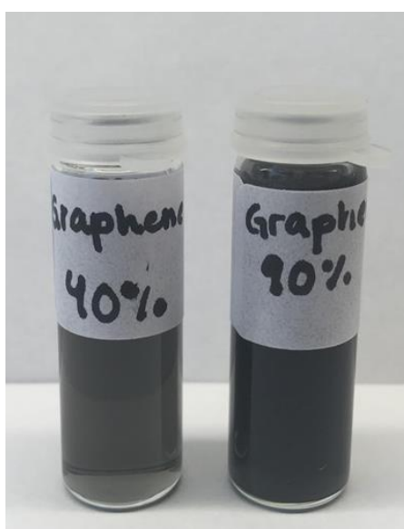
Figure 2.3: Graphene prepared in a tip sonicator in icebath for 30 min at respectively 28 Watt (40 %) and 63 Watt (90 %).
