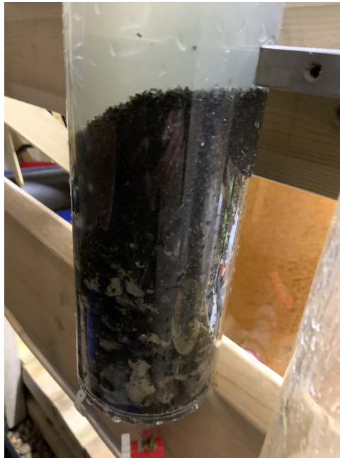
Figure 3.14: Activated carbon on top of gravel in the pipe setup at Killingdal.
