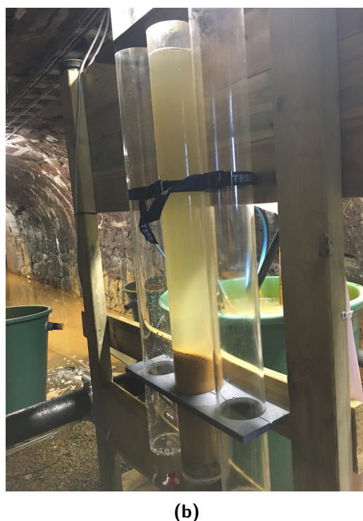
Figure 3.13: Removal efficiency of the trace elements in focus by activated carbon was tested on site at Killingdal. Figure 3.13a shows how the setup was initially planned to be. Figure 3.13b shows what the actual setup used at Killingdal looks like.
