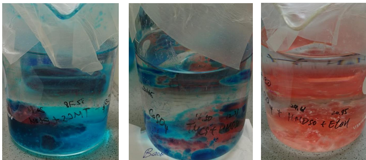
Figure 5.2. Pictures were taken 10 minutes after gel immersed in surface modifying solutions. (left) S(II)-T: The gel immersed in a solution containing TMCS and n-heptane/EtOH, (middle) S(II)-T/H: The gel immersed in a solution containing mixture of TMCS/HMDSO and n-heptane/EtOH (right) S(II)-H: The gel immersed in a solution containing HMSDO and n-heptane/EtOH
