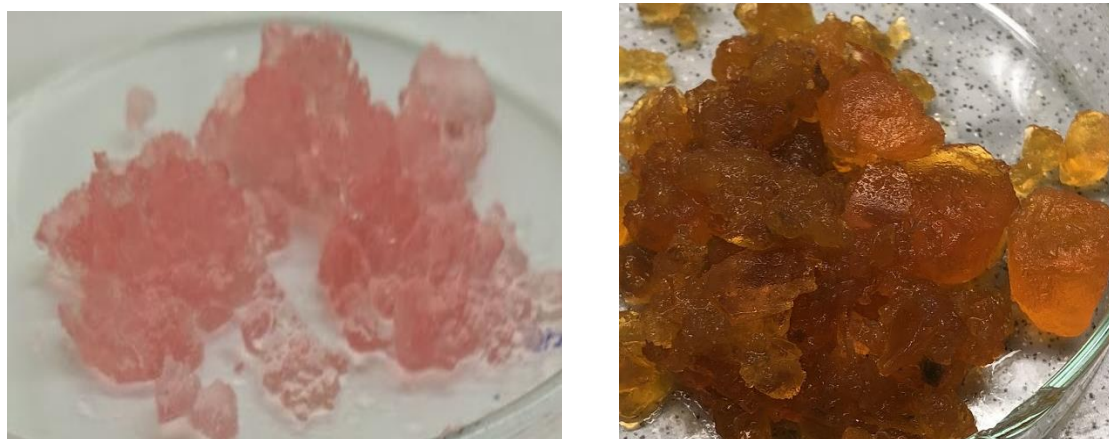
Figure 5.1. Picture was taken after aging and before surface modification. ( left ) S(II)-H: Gel prepared using \text{CoSO}_4 as cobalt precursor. ( right ) A(III)-H: Gel prepared using [\text{Co}(\text{NH}_3)_6]\text{Cl}_3 as cobalt precursor.
