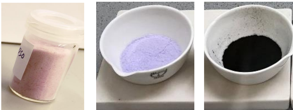
Figure. 5.6. Colour of S_C 6 _60C powder sample hydrophobized at 60°C in modifying solvents of HMDSO and n-heptane/ EtOH: as prepared ( left ), annealed ( middle ) and calcined ( right ).
