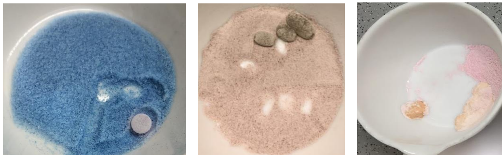
Figure. 5.4. Pictures show hydrophobicity of samples. (left) S(II)-T (middle) S(II)-T/H (right) S(II)-H
