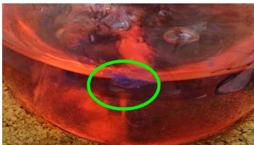
Figure. 5.5 Addition of Ammonium hydroxide to sol led to the formation of blue coagula (green circle) in the gel.
