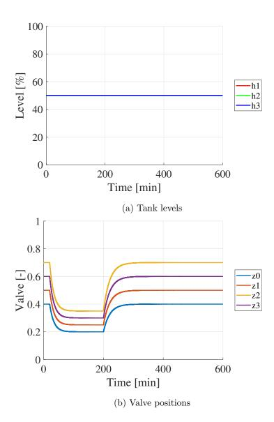
Figure 22: Disturbance on  $z_3$  with MPC. The MPC is given the information that from t = 20 minutes z3 is the desired TPM with a desired value of 0.3, until at t = 200 where z0 is the TPM again with a desired value of 0.4.
