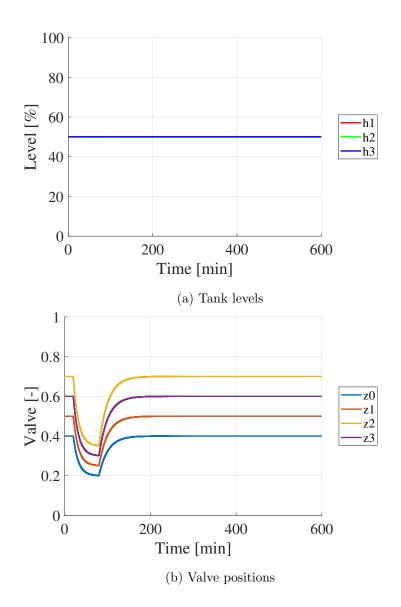
Figure 26: Disturbance on  $z_2$  with MPC. The MPC is given the information that from t = 20 minutes z2 is the desired TPM with a desired value of 0.35, until at t = 200 where z0 is the TPM again with a desired value of 0.4.
