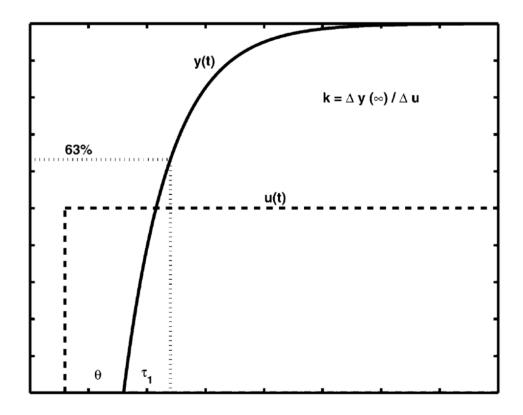
Figure 2: Open-loop step response of a first-order process with a time delay  $\theta$  and time constant  $\tau_1$ . u is the controller output and y is the controlled variable. Figure retrieved from [15].
