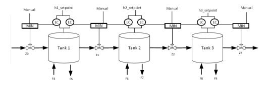
Figure 16: Control structure with generalized split range control. The two level controllers are split up with additional logic (not shown) to prevent unwanted switching, as they have the same setpoint.
