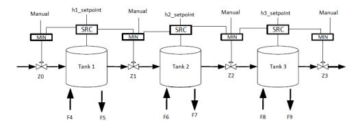
Figure 15: Control structure for the modeled process with split range control.
