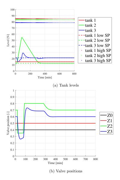
Figure 23: Disturbance on  $z_2$  for control structure with two controllers with different setpoints. The manual input for  $z_2$  is reduced from 1 (inactive) down to 0.35 at t = 20 minutes becoming the active input, and later raised to 0.8 where it becomes a temporary bottleneck before the system settles back to the nominal point.
