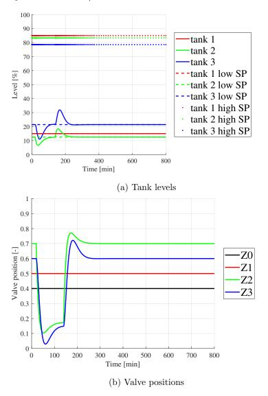
Figure 34: External draining of tank 2 with a flow (F7) of 0.12  $m^3/min$  from t = 20 to t = 140 minutes with two controllers for each tank.
