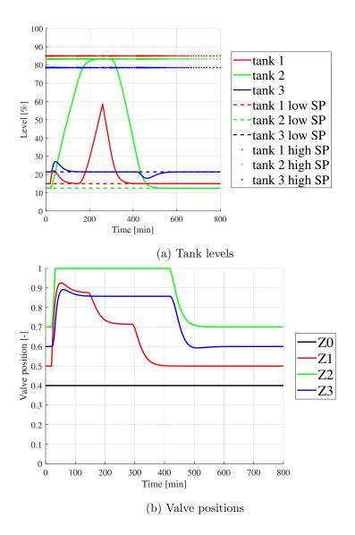
Figure 31: External filling of tank 1 with a flow (F4) of 0.12  $m^3/min$  from t = 20 to t = 260 minutes with two controllers for each tank.
