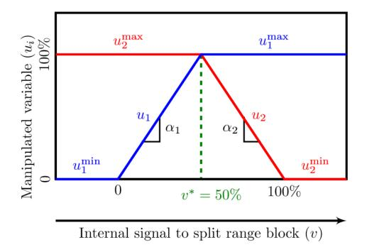
Figure 5: Split range block, with the split value  $v^*$  at the midpoint (50%). Figure retrieved from [11].
