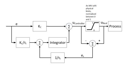
Figure 11: PI controller with back calculation. An MV has physical limits, but a controller does not. When there is a difference between the controller output and the value of the MV ( $e_s \neq 0$ ) this value is multiplied with  $1/\tau_t$  and added to the integrator, resetting the controller dynamically.
