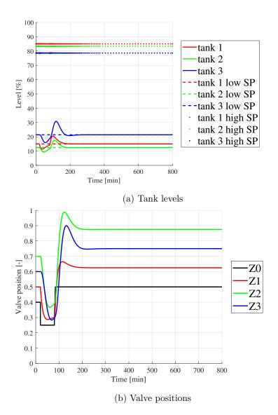
Figure 27: Disturbance on  $z_0$  for control structure with two controllers with different setpoints. The manual input for  $z_0$  is reduced from 1 (inactive) down to 0.25 at t = 20 minutes becoming the active input, and later raised to 0.5
