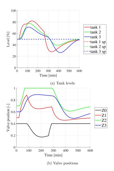
Figure 32: External filling of tank 1 with a flow (F4) of 0.12  $m^3/min$  from t = 20 to t = 260 minutes with split range control
