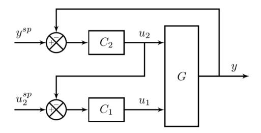
Figure 7: Valve position control structure where two MVs are used to control one CV. The MV  $u_2$  controls the CV y, while the MV  $u_1$  is used to control  $u_2$ back to a desired setpoint. Figure retrieved from [9].
