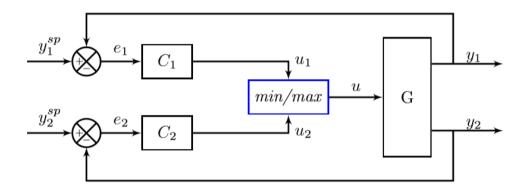
Figure 9: Min- or max-selector. Figure retrieved from [9].
