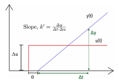
Figure 3: Open-loop step response for an integrating process with gain k', y is the CV, u is the MV and  $\theta$  is the time delay. Figure retrieved from [16].
