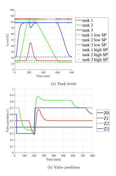
Figure 19: Disturbance on  $z_3$  for control structure with two controllers with different setpoints. The manual in-put for z3 is reduced from 1 (inactive) down to 0.3 at t = 20 minutes becoming the active input, and at t = 200 minutes raised to 0.7 where it becomes a temporary bottleneck before the system settles back to the nominal point.
