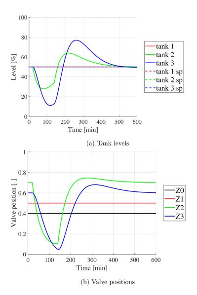
Figure 35: External draining of tank 2 with a flow (F7) of 0.12  $m^3/min$  from t = 20 to t = 140 minutes with split range control.
