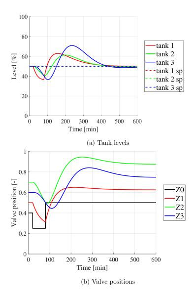
Figure 28: Disturbance on  $z_0$  with split range control. The manual input for  $z_0$  is reduced from 1 (inactive) down to 0.25 at t = 20 minutes becoming the active input, and later raised to 0.5
