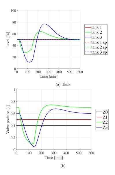
Figure 36: External draining of tank 2 with a flow (F7) of 0.12  $m^3/min$  from t = 20 to t = 140 minutes with generalized split range control.
