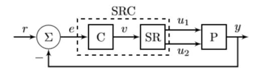
Figure 6: Split range controller. The CV y is controlled with the two MVs  $u_1$  and  $u_2$ . Figure retrieved from [11].
