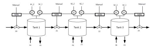
Figure 17: Control structure for the modeled process with two controllers with different setpoints.
