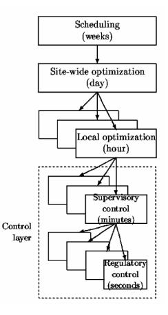
Figure 4: Control hierarchy in a chemical plant, separated into layers by different time scales. Figure retrieved from [14].
