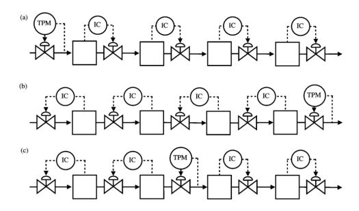
Figure 1: Consistent inventory control, to ensure that the steady-state mass balance is fulfilled. Figure retrieved from [3].
