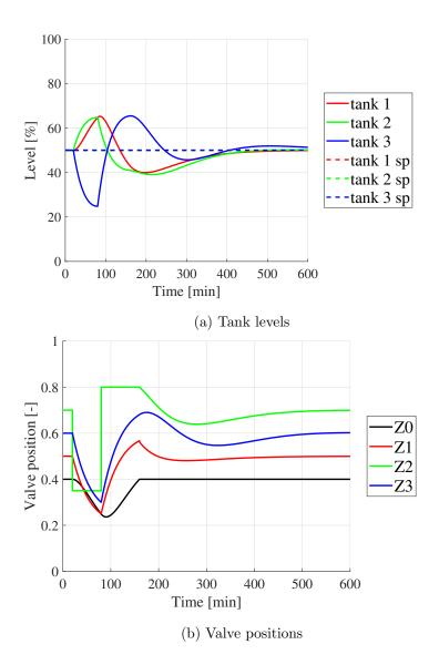
Figure 25: Disturbance on  $z_2$  with generalized split range control. The manual input for  $z_2$  is reduced from 1 (inactive) down to 0.35 at t = 20 minutes becoming the active input, and later raised to 0.8 where it becomes a temporary bottleneck before the system settles back to the nominal point.
