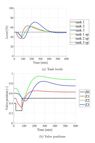
Figure 29: Disturbance on  $z_0$  with generalized split range control. The manual input for  $z_0$  is reduced from 1 (inactive) down to 0.25 at t = 20 minutes becoming the active input, and later raised to 0.5
