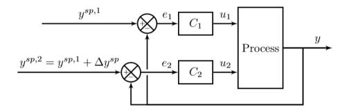
Figure 8: Controllers for different MVs with different setpoints for the same CV. A difference  $\Delta Y^{sp}$  is needed to let only one controller be active at a given point in time. Figure retrieved from [9].
