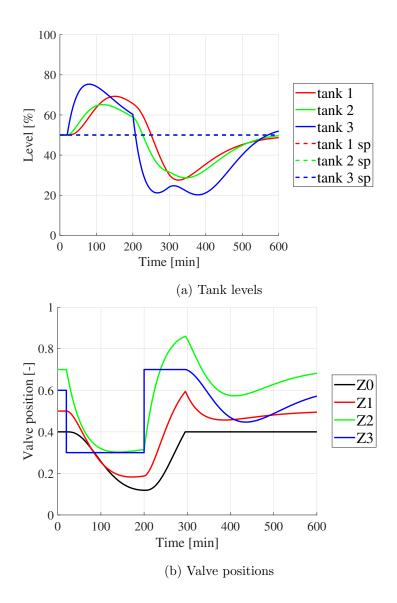
Figure 20: Disturbance on the outlet  $(z_3)$  with split range control. The manual input for z3 is reduced from 1 (inactive) down to 0.3 at t = 20 minutes becoming the active input, and at t = 200 minutes raised to 0.7 where it becomes a temporary bottleneck before the system settles back to the nominal point.
