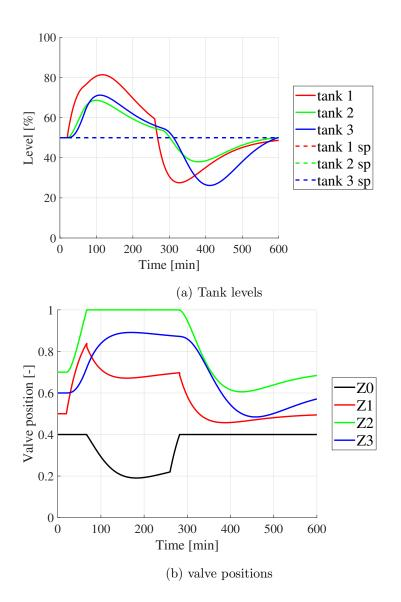
Figure 33: External filling of tank 1 with a flow (F4) of 0.12  $m^3/min$  from t = 20 to t = 260 minutes with generalized split range control
