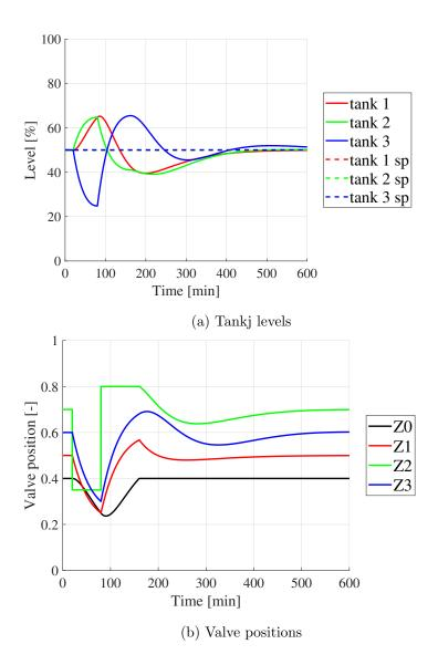
Figure 24: Disturbance on  $z_2$  with split range control. The manual input for  $z_2$  is reduced from 1 (inactive) down to 0.35 at t = 20 minutes becoming the active input, and later raised to 0.8 where it becomes a temporary bottleneck before the system settles back to the nominal point.
