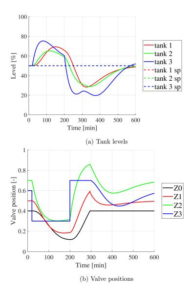
Figure 21: Disturbance on  $z_3$  with generalized split range control. The manual input for z3 is reduced from 1 (inactive) down to 0.3 at t = 20 minutes becoming the active input, and at t = 200 minutes raised to 0.7 where it becomes a temporary bottleneck before the system settles back to the nominal point.
