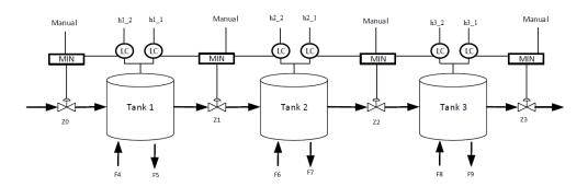
Figure 14: Control structure with additional disturbances (inflows and outflows).
