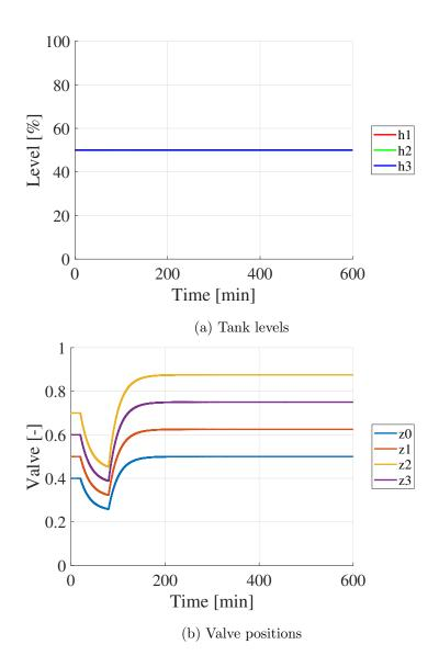
Figure 30: Disturbance on  $z_0$  with MPC. The MPC is given the information that from t = 20 minutes the desired value of z0 is 0.25, and after t = 200 the desired value is 0.5.
