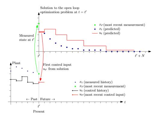
Figure 12: Principle of how an MPC works. x denotes the CV, while u denotes the MV. Figure retrieved from [7].
