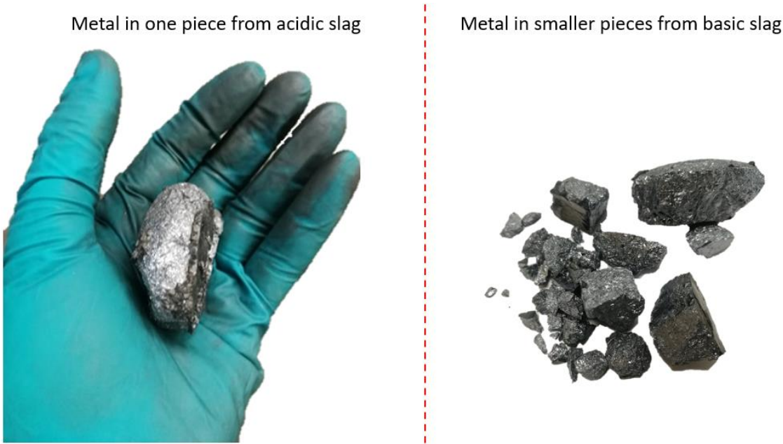
Figure 4.17: Main metal lump separated form (parallel 3) acidic slag and stoichiometric reduction amount (left). Metal pieces comprising the metal yield form (parallel 3) basic slag and stoichiometric reductant amount, after separation (right).
