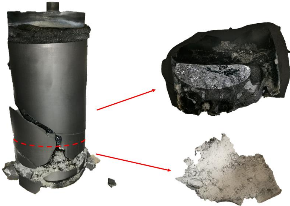
Figure 4.19: Cacked crucible after experiment conducted with basic master slag. Illustrate grey powder found in bottom off all experiments with basic slag, as well as the cross section of metal and slag form this parallel.
