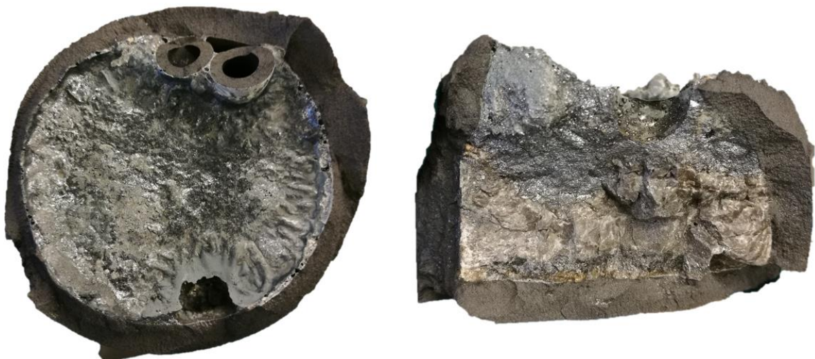
Figure 4.21: 1. Parallel of acidic slag with 1.1*stoichiometric Al amount: illustrate the top (left), and cross section of the sample. The metal had not coalesced in this sample, there were instead a dense dispersion of metal droplets in the top half of the slag.
