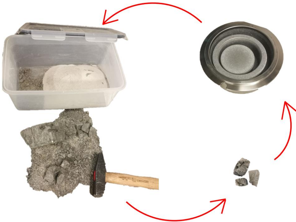
Figure 3.3: Illustrating how slag was crushed down to smaller pieces with a hammer, the tungsten carbide discs used for the crushing, and the resulting slag powder.
