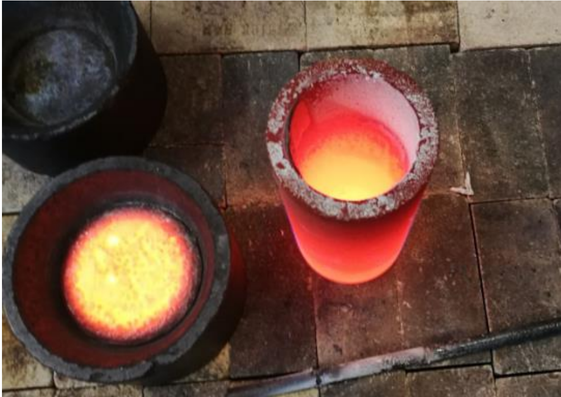
Figure 3.2: Crucible, cast and the slag produced ( \text{CaO}/\text{SiO}_2 ) directly after casting
