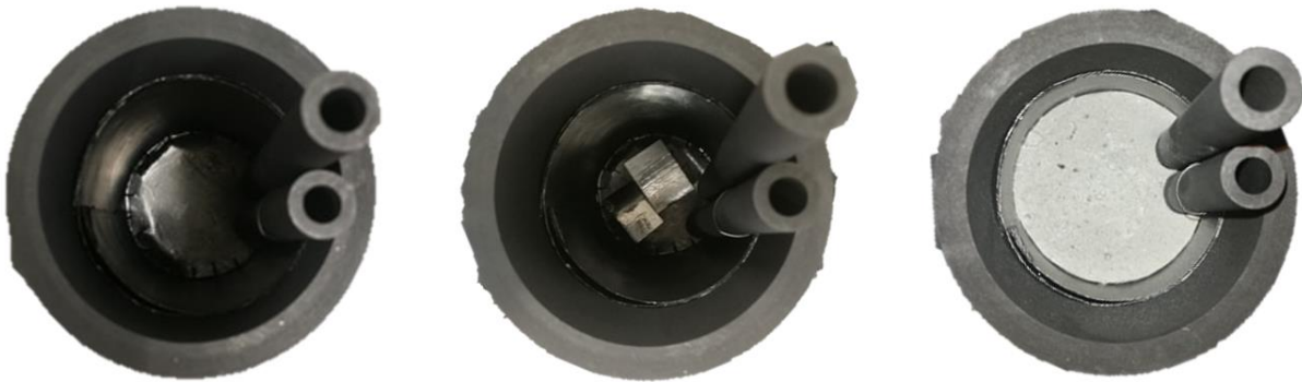
Figure 3.7: Illustrate the charging process with empty crucible (left), charged with the Al used as reductant (middle), and charged with slag on top of the reductant (right). (NB! The graphite paper observed inside the crucible was tested out, but not used for the experiments described here due to problems that arose when used)
