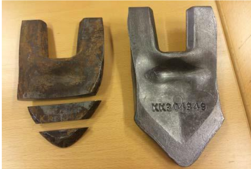
Figure 2-4 Differences in dimensions between a worn and new tine point [19].
