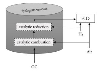
Figure 2-6 Schematic view of the Polyarc reactor, inspired by Jones at ARC [10].
