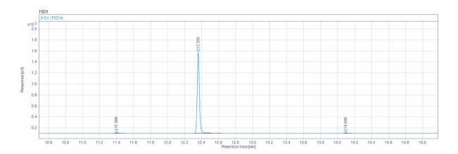
Figure 4-17 Chromatogram for sample D1 with 99% purity, extra column gradient method 1.
