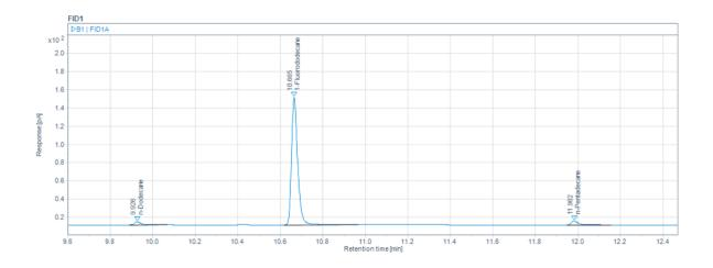
Figure 4-3 Chromatogram for sample B1 with 95% purity.
