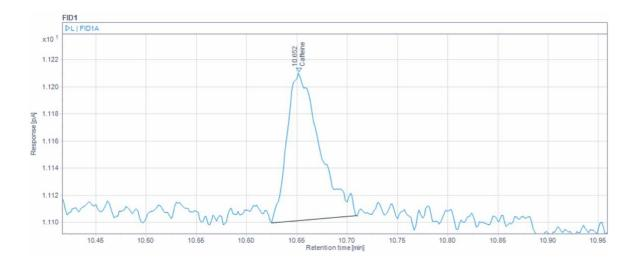
Figure 4-13 Chromatogram for sample L (0,98  $\mu$ g/mL) from linearity test. S/N = 10.5.
