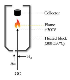
Figure 2-5 Schematic view of the flame ionization detector, inspired by Lundanes et al. [8].
