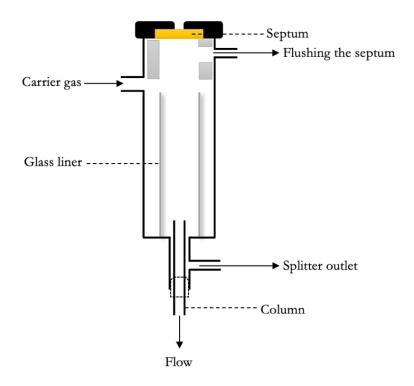
Figure 2-2 Illustration of a split/splitless injector, inspired by Lundanes et al. [8].
