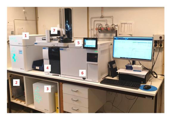
**Figure 3-1** Overview of the GC. (1) Air and H<sub>2</sub> generators, (2) vacuum pump for MSD, (3) air compressor, (4) MSD, (5) Polyarc/FID, (6) column oven, (7) autosampler. Photo: Stine Rapp.
