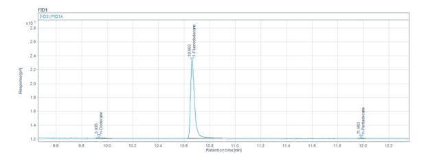
Figure 4-15 Chromatogram for sample D3 with 99% purity (diluted x10).
