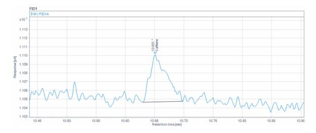
Figure 4-14 Chromatogram for sample M (0,49  $\mu$ g/mL) from linearity test. S/N = 5.2.
