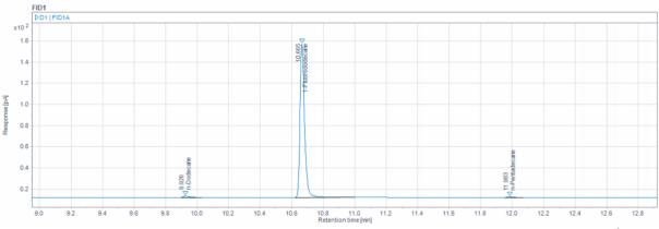
Figure 4-19 Chromatogram for sample D1 with 99% purity, original injector temp. (250°C).
