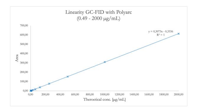
Figure 4-7 Linearity results of caffeine for peak areas from GC/Polyarc-FID.
