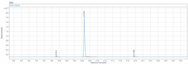
Figure 4-20 Chromatogram for sample D1 with 99% purity, extra injector temp. 1 (245°C).
