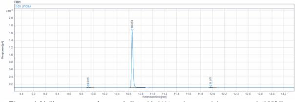
Figure 4-21 Chromatogram for sample D1 with 99% purity, extra injector temp. 2 (255°C).
