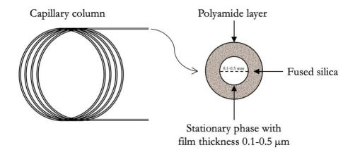
Figure 2-3 Illustration of a WCOT fused silica capillary column, inspired by Lundanes et al. [8].
