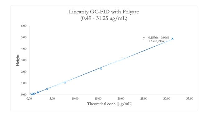
Figure 4-10 Linearity results of caffeine for peak heights of a smaller range for the Polyarc-FID.
