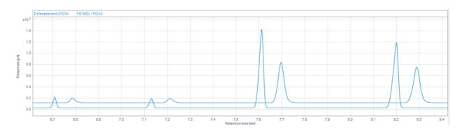
**Figure 5-1** Chromatogram of a checkout sample analyzed with and without a Polyarc, where the tallest and narrowest peaks are results from Polyarc-FID.
