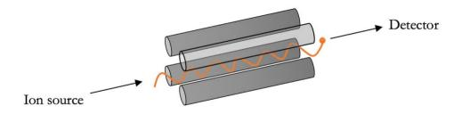
Figure 2-4 Illustration of the quadrupole, inspired by Lundanes et al. [8].
