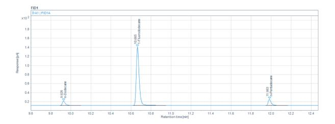
Figure 4-2 Chromatogram for sample A1 with 90% purity.
