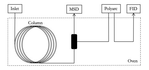
Figure 2-1 Schematic view of a GC-MS with a Polyarc-FID, inspired by Jones at ARC [10].
