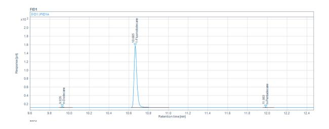
Figure 4-5 Chromatogram for sample D1 with 99% purity.
