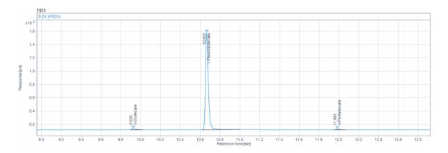
Figure 4-16 Chromatogram for sample D1 with 99% purity, original column gradient method.
