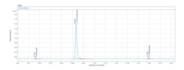
Figure 4-4 Chromatogram for sample C1 with 97% purity.
