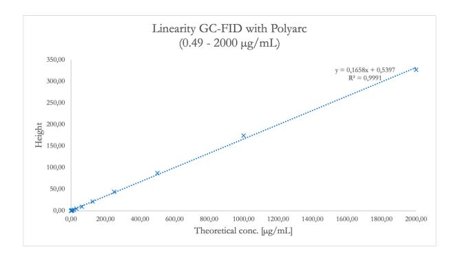
Figure 4-9 Linearity results of caffeine for peak heights from GC/Polyarc-FID.
