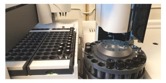
Figure 3-2 The 7693A autosampler, with the ability to load 150 samples. Photo: Stine Rapp.
