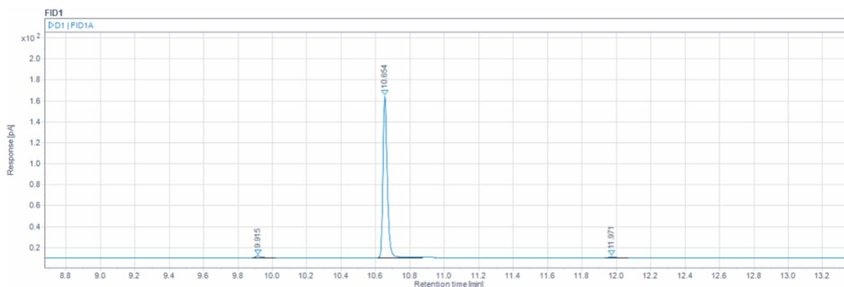
**Figure 4-21** Chromatogram for sample D1 with 99% purity, extra injector temp. 2 (255°C).
