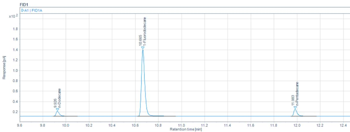
Figure 4-2 Chromatogram for sample A1 with 90% purity.
