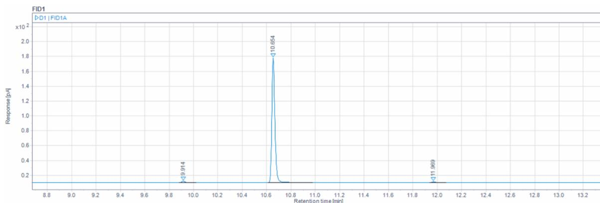
**Figure 4-20** Chromatogram for sample D1 with 99% purity, extra injector temp. 1 (245°C).
