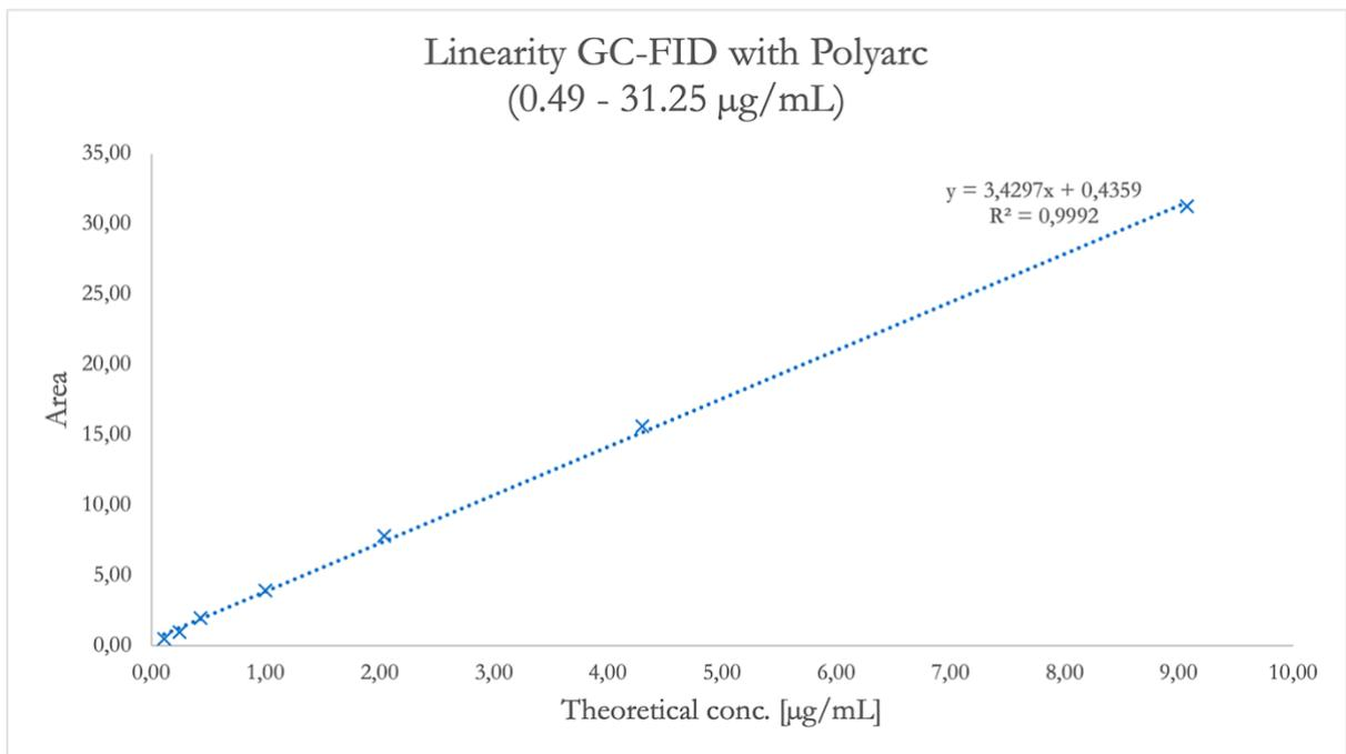
**Figure 4-8** Linearity results of caffeine for peak areas of a smaller range for the Polyarc-FID.
