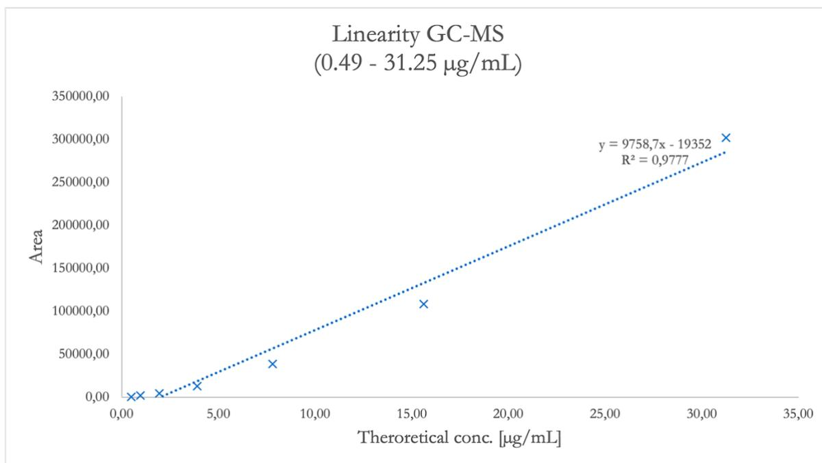
**Figure 4-12** Linearity results of caffeine for peak areas of a smaller range for the MS.
