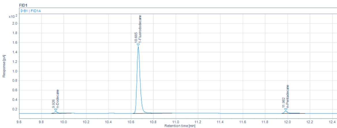
Figure 4-3 Chromatogram for sample B1 with 95% purity.
