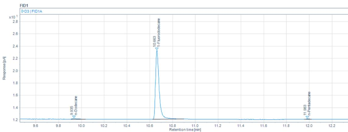
**Figure 4-15** Chromatogram for sample D3 with 99% purity (diluted  $\times 10$ ).
