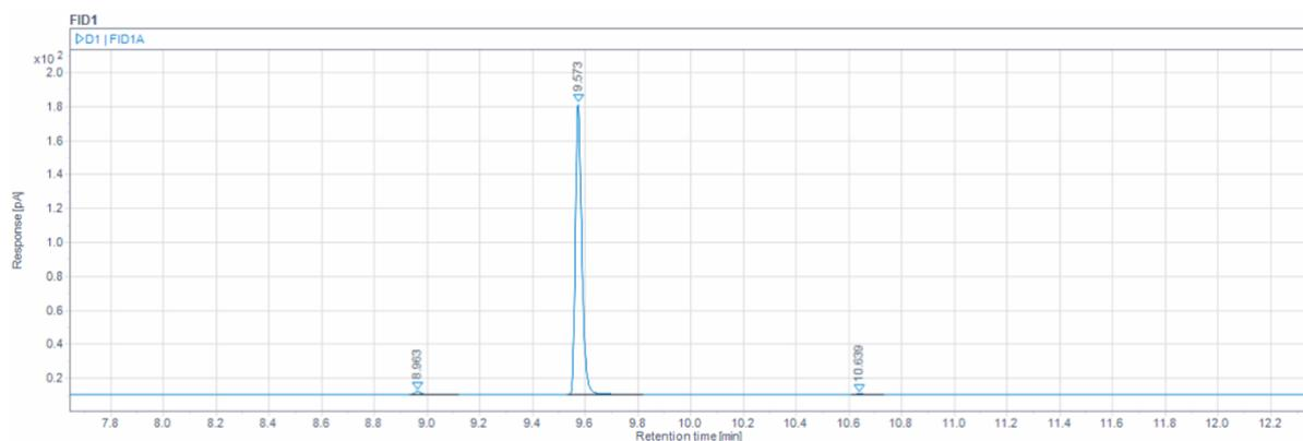
**Figure 4-18** Chromatogram for sample D1 with 99% purity, extra column gradient method 2.
