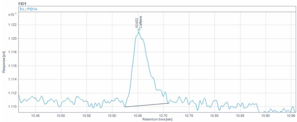
**Figure 4-13** Chromatogram for sample L ( $0,98 \mu\text{g}/\text{mL}$ ) from linearity test.  $S/N = 10.5$ .
