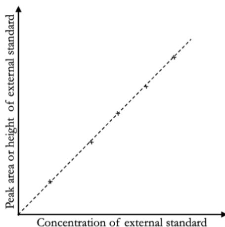
**Figure 2-8** Calibration curve for an external standard.
