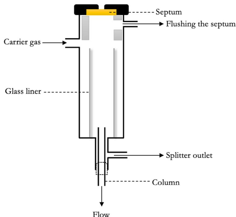
**Figure 2-2** Illustration of a split/splitless injector, inspired by Lundanes et al. [8].
