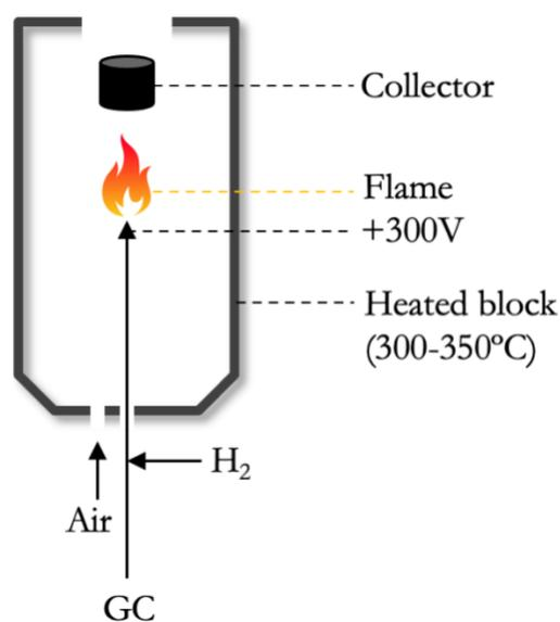
**Figure 2-5** Schematic view of the flame ionization detector, inspired by Lundanes et al. [8].
