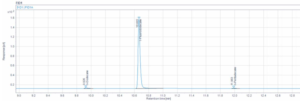
**Figure 4-16** Chromatogram for sample D1 with 99% purity, original column gradient method.
