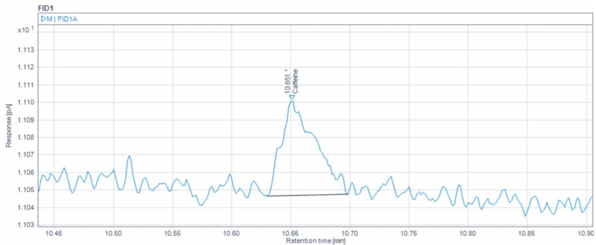
**Figure 4-14** Chromatogram for sample M ( $0,49 \mu\text{g}/\text{mL}$ ) from linearity test.  $S/N = 5.2$ .
