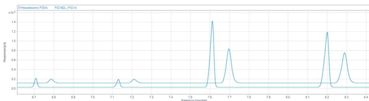
**Figure 5-1** Chromatogram of a checkout sample analyzed with and without a Polyarc, where the tallest and narrowest peaks are results from Polyarc-FID.
