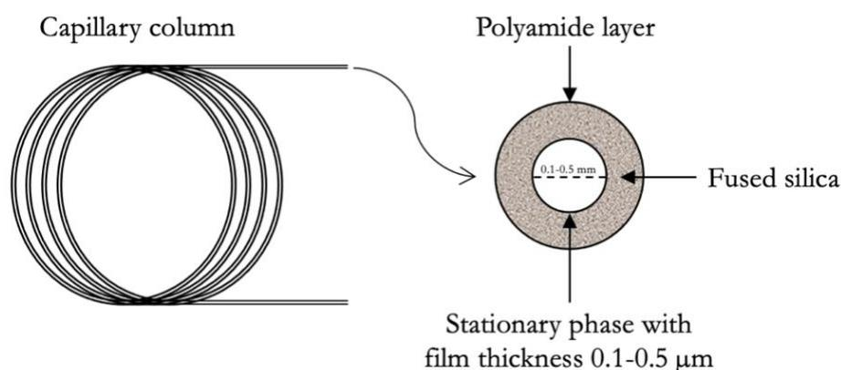
**Figure 2-3** Illustration of a WCOT fused silica capillary column, inspired by Lundanes et al. [8].
