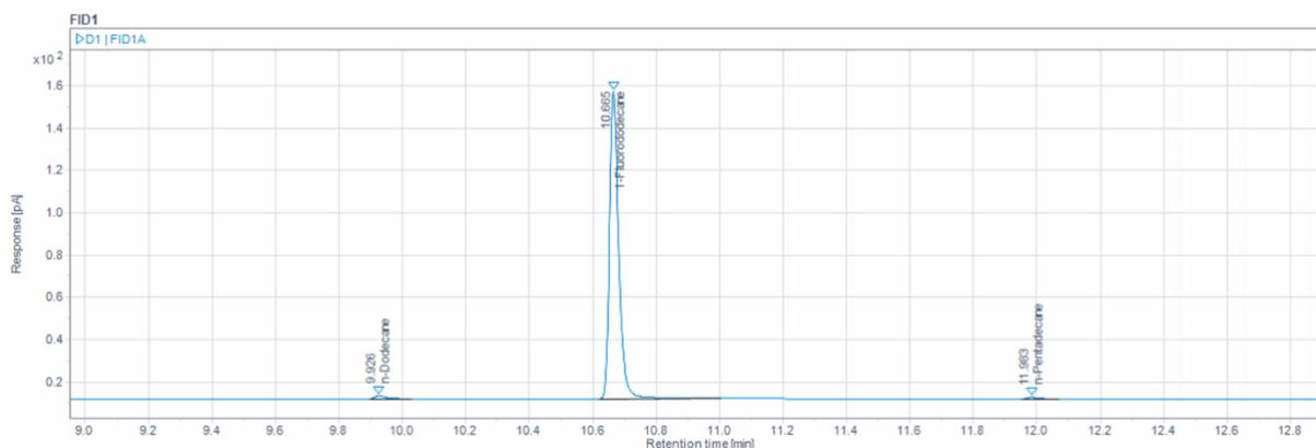
**Figure 4-19** Chromatogram for sample D1 with 99% purity, original injector temp. (250°C).
