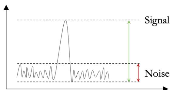
Figure 2-9 Illustration of the definitions signal and noise.
