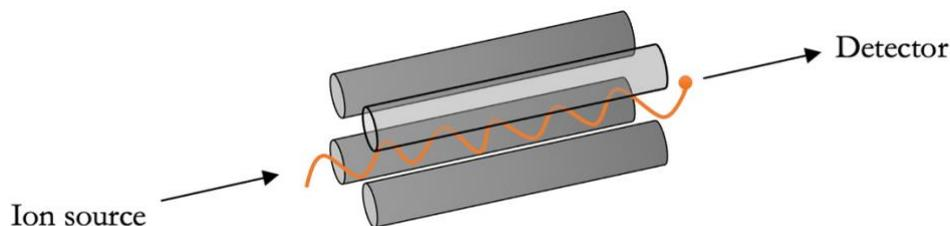
**Figure 2-4** Illustration of the quadrupole, inspired by Lundanes et al. [8].
