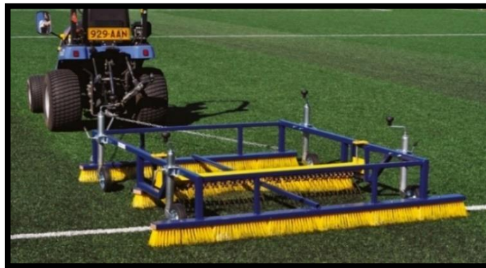
Figure 2. Example of how a brush for artificial turf could look. These are generally attached to a vehicle (26).
