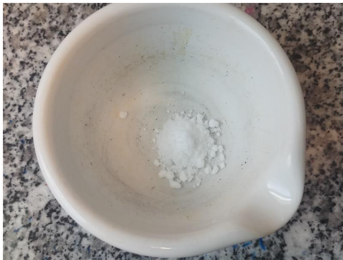
Figure 2.5 – Image of recrystallized NIPAM.
