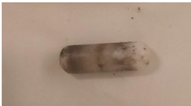
Figure 4.1 – Image of magnetic stirrer showing sticking problem, when phase transferred particles (4.7 mg) was used during in situ reaction.
