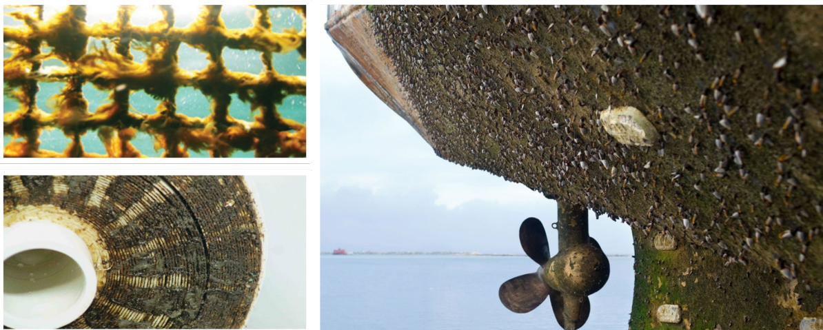
Figure 1.1: Captions of biofouling from maritime industries. The pictures visualize fouling on fish nets (top left), membrane (bottom left) and vessel hull (right). Images are modified from [2, 3, 4]
