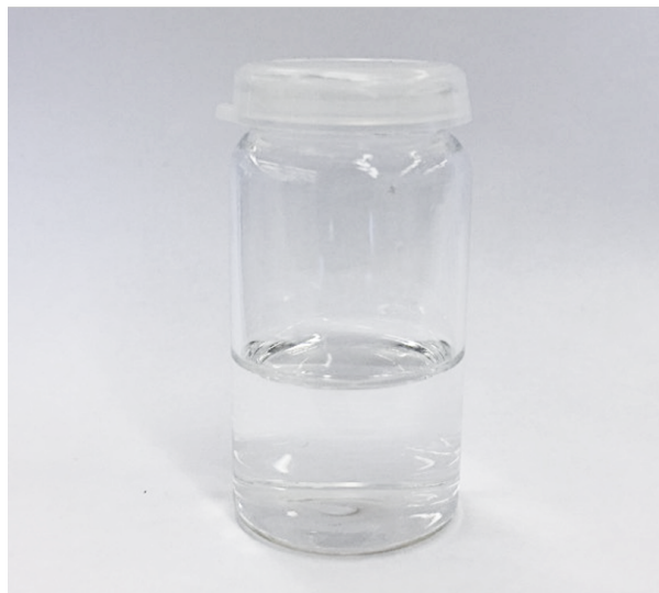
Figure 4.2: Caption of synthesized silica sol. No change in visual appearance was observed over time.
