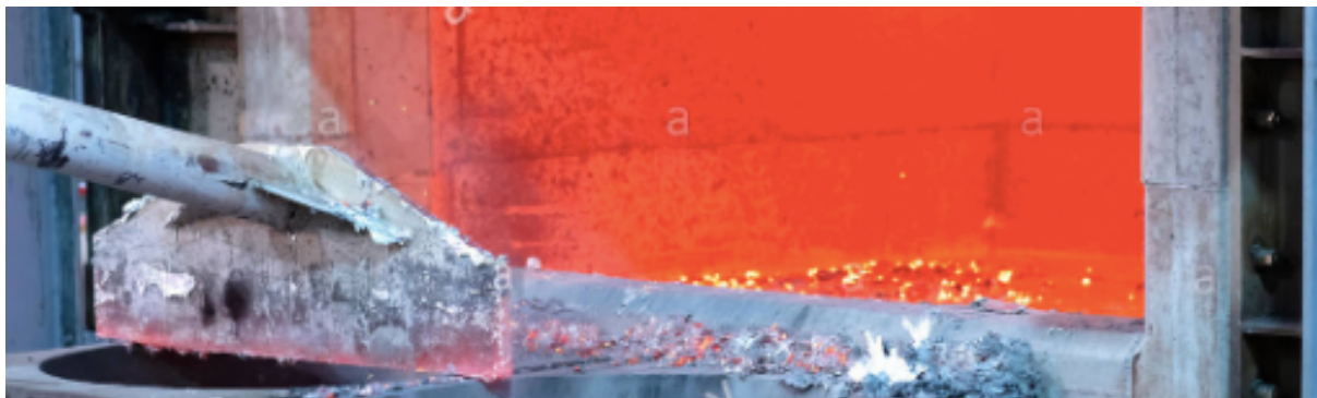
Figure 2.21. Example of dross skimming operation.
