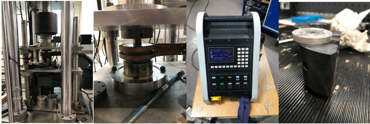
Figure 3.10. The equipment for pressing with induction and the briquette produced.
