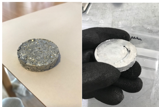
Figure 3.12. Images showing the surface irregularities of briquette compressed uniaxially (left) and HPT (right).
