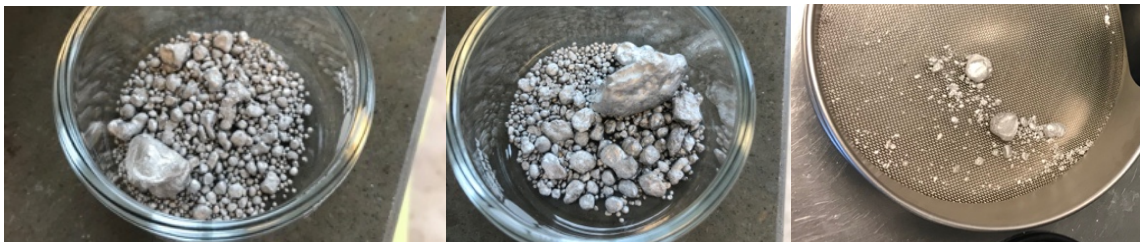
Figure 4.28. The recovered Al of briquettes corresponding to column 1, 2 and 4 in Table 4.5 above.
