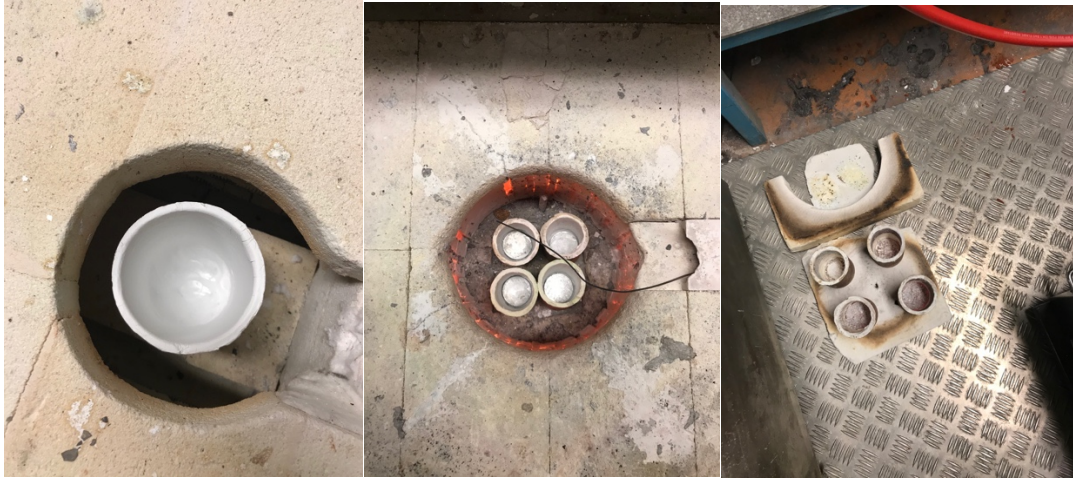
Figure 3.18. Dried crucible (left), charged crucible with briquettes inside (middle) and finished heated briquettes (right).
