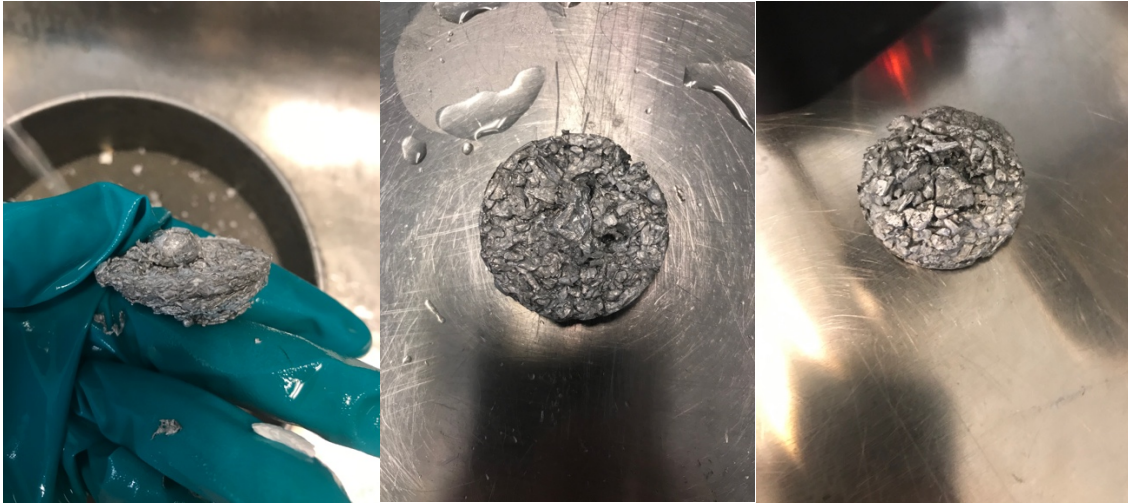
Figure 4.37. Unsuccessful coalescence of briquettes with approximate bulk density 2.1 \text{ g/cm}^3 . 100, 200 and 300 \mu\text{m} , from left to right.
