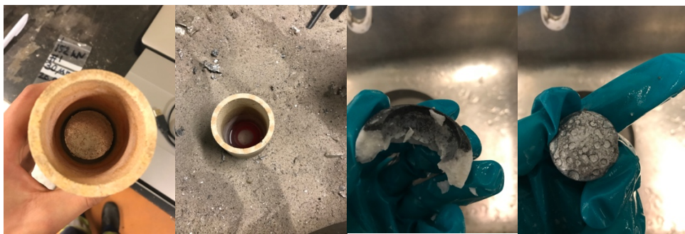
Figure 3.16. Crucible with solid and molten briquette, salt flux after operation and coalesced aluminum.
