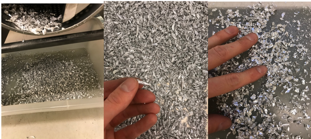
Figure 3.4. Chips that passed and were collected by the screen, deformed chips and undeformed chips.
