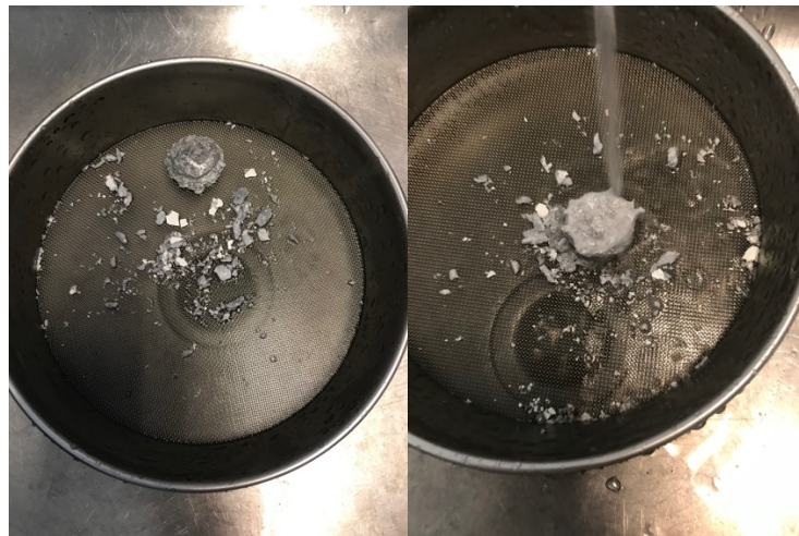
Figure 4.36. Unsuccessful coalescence of briquettes with approximate bulk density 2.1 g/cm 3 . 15 and 30 \mu\text{m} , from left to right.
