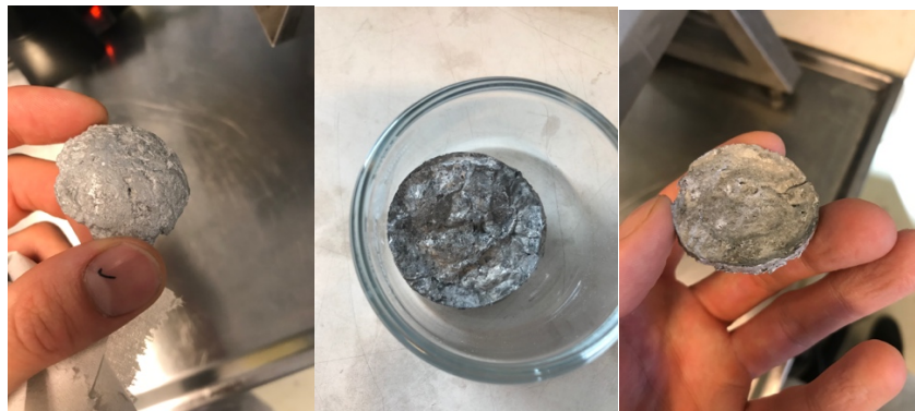
Figure 4.38. Briquettes of 15, 100 and 200 \mu\text{m} , with bulk density 2.6, 2.5 and 2.5 \text{ g/cm}^3 , respectively.
