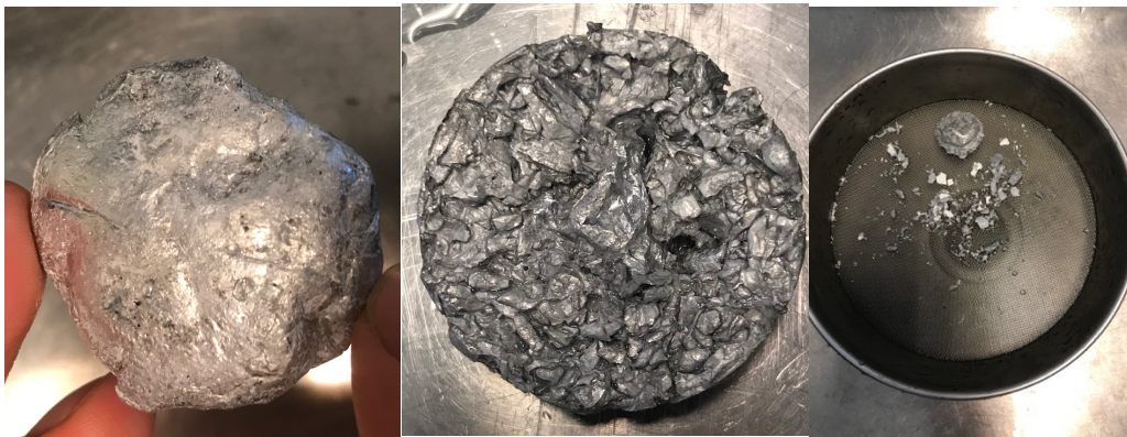
Figure 3.19. Successfully recovered Al (left), visible chips (middle) and fragile Al piece disintegrating (right).
