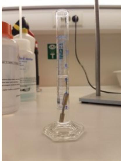
Figure 19: Setup for the density measurements using Archimedes' principle.
