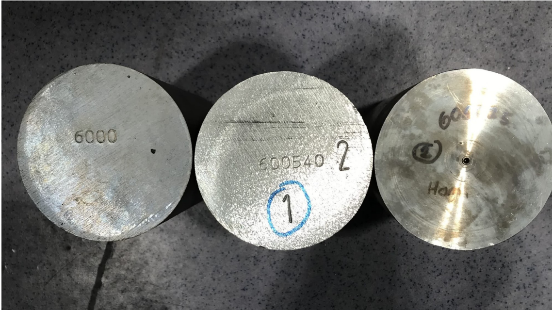
Figure 3.2: Billets in the 6xxx series. The billet to the left labelled 6000 is the 6082 billet. The middle and right billet is 6005.40 and 6060.35, respectively.
