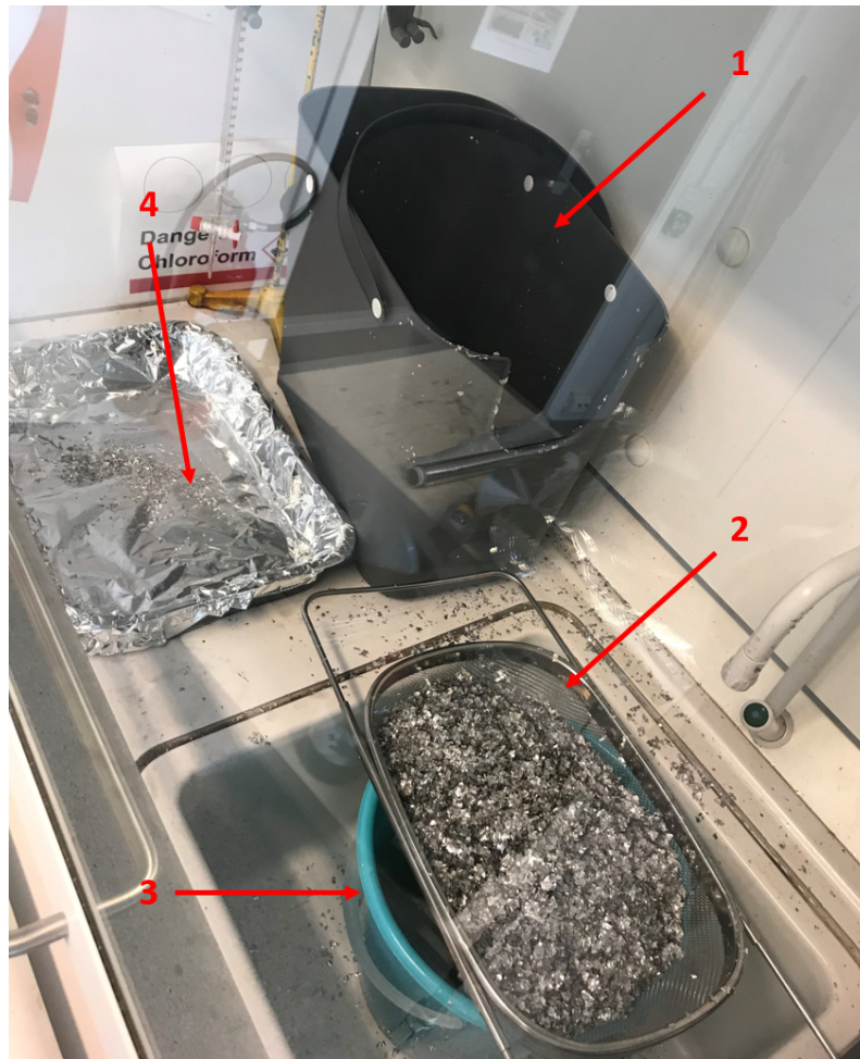
Figure 3.4: Acetone degreasing equipment. 1) - PP waste container for degreasing granules with acetone; 2) - 5 mm mesh sieve for screening acetone out of the granules; 3) - 10 L PP bucket for collecting screened acetone; 4) - Al-foil covered tray for acetone degreased granules.
