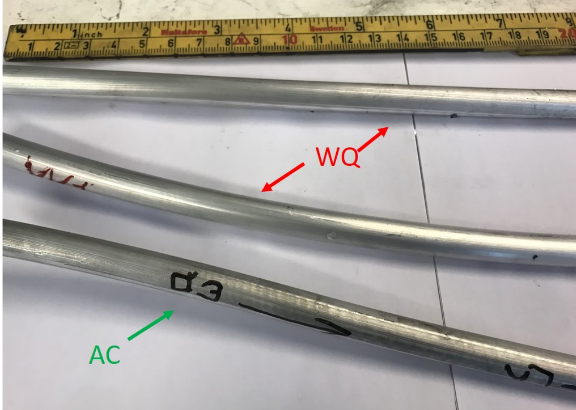
Figure 4.7: A section of the screw extruded 6082 profiles. The two on the top are water quenched (WQ) and the bottom profile is air cooled (AC).
