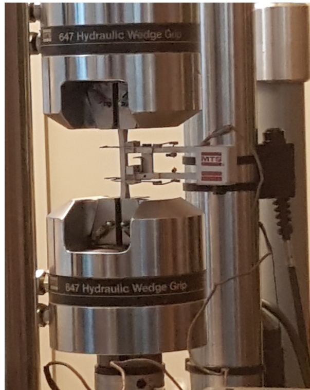
Figure 3.6: Sample in a 110kN test machine[2].
