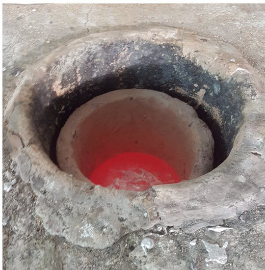
Figure 3.1: Melted aluminium in induction oven[2].
