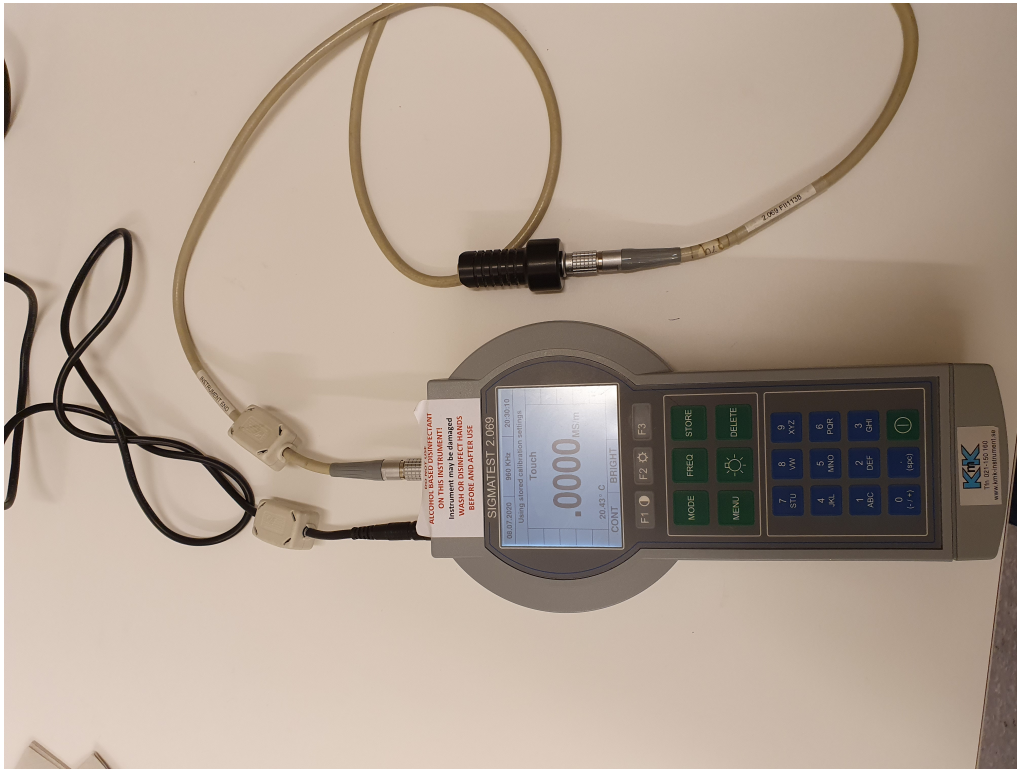
Figure 3.8: Sigmatess 2.069 apparatus used to calculate electrical conductivity.
