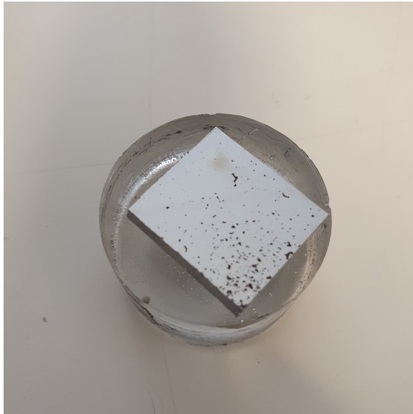
Figure 3.7: Example of sample after polishing and ready for hardness testing.
