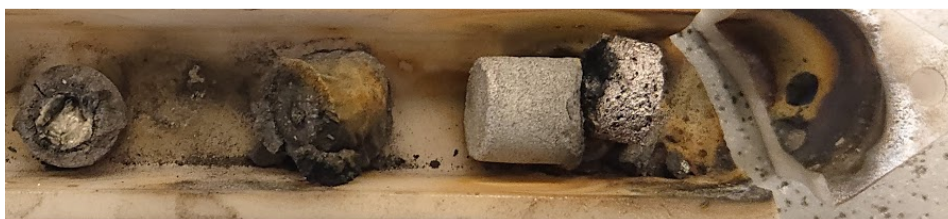
Figure D6: Images of Samples Zr+2Si(600 °C, Ign. in cylinder) and Zr+2Si(600 °C, Ign. in cylinder) a) before and b) after the experiment
