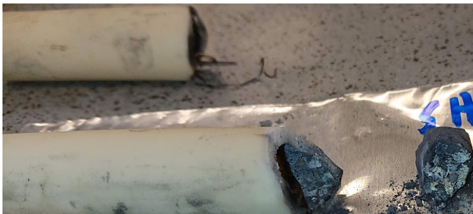
Figure D4: Image of alumina tube sample container and part of Zr+2Si beam that was in contact with igniter during a room temperature SHS experiment where the filament was adjacent to the igniter pellet which was in contact with the Zr+2Si beam
