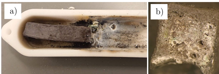
Figure D3: Images of the sample Zr+2Si(Room temp, Indep. Ign)1 (see Table 3.5). a) is a top view of the sample, and b) is an image of the side that was in contact with the igniter
