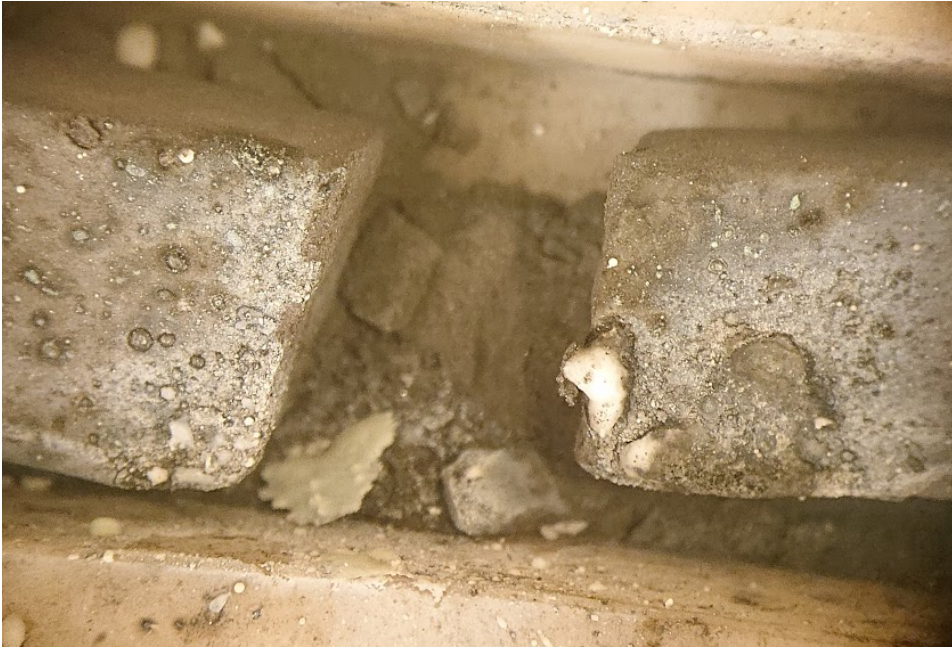
Figure D5: Zr+Si(Room temp, Ign. in fila.) (see Table 3.5) after experiment. The small white pieces are pieces of the exploding igniter.
