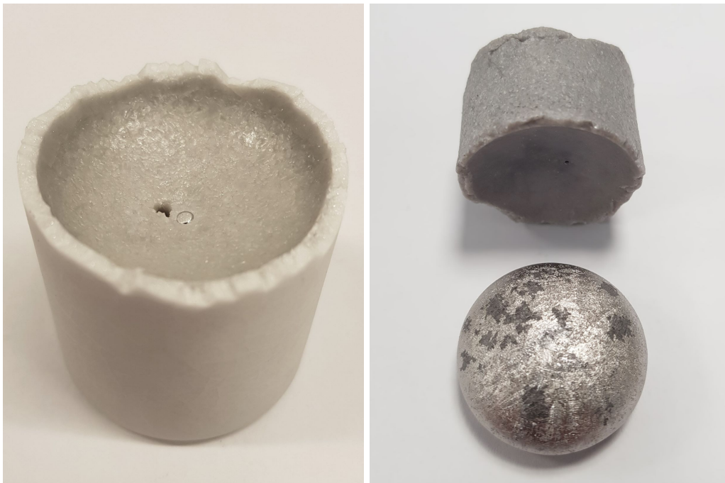
(a) The top of the slag after removing the upper part of the crucible. (b) The slag and metal after removing the crucible.
