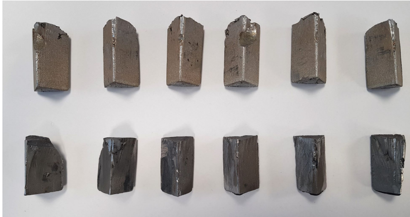
Figure 3.7: The pieces of the master alloys as received from the workshop. The upper pieces are MA1 and the lower pieces are MA2. The rust visible on the MA1 pieces developed during the laboratory lockdown.
