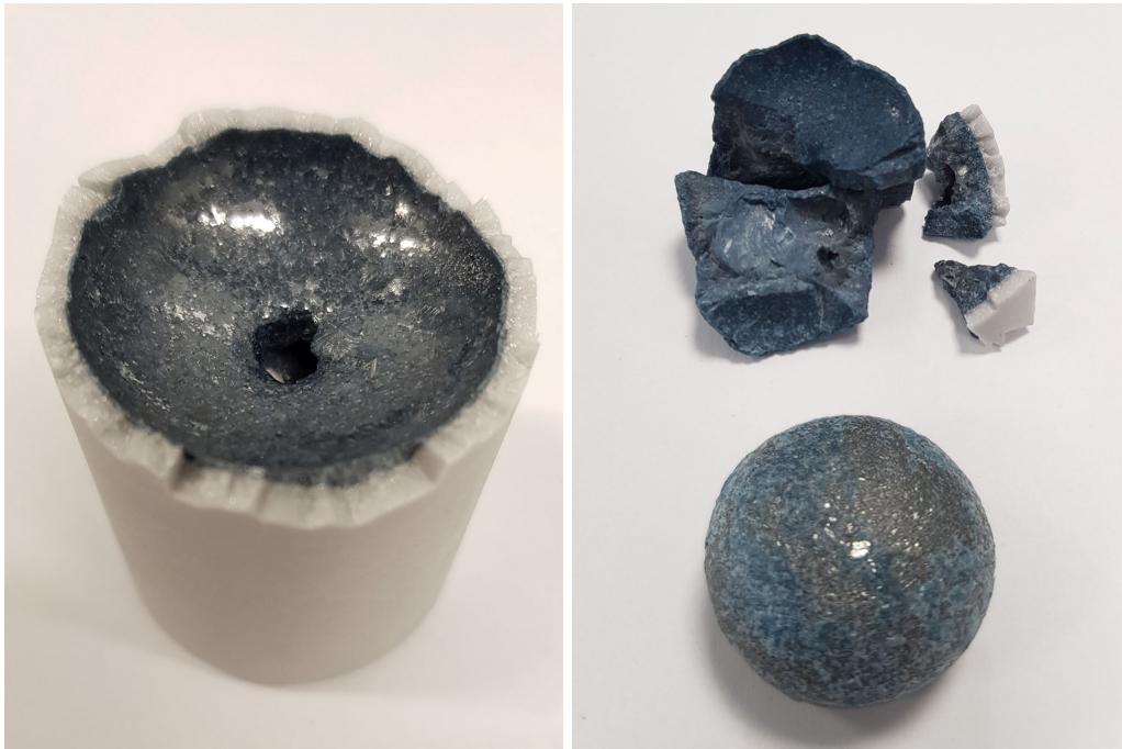
(a) The top of the slag after removing the upper part of the crucible. (b) The slag and metal after crushing and removing the slag from the larger parts.
