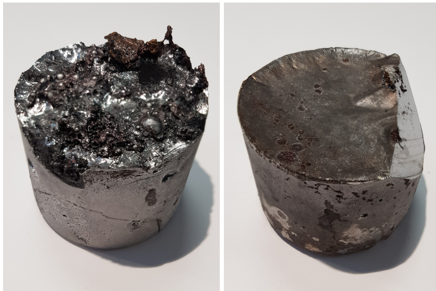
(a) The 1% Ti alloy (MA1) before cutting. (b) The 3% Ti alloy before (MA2) cutting.
