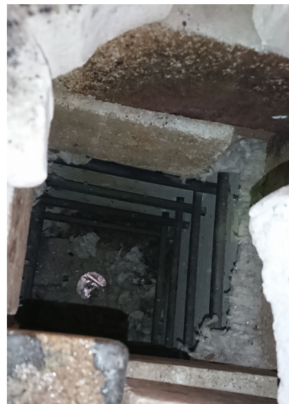
(b) The inside of the furnace. Carbon rods were used at heating elements,
