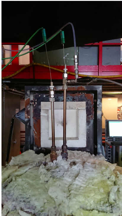
(a) Thermocouples and off-gas collection for the exhaust.
