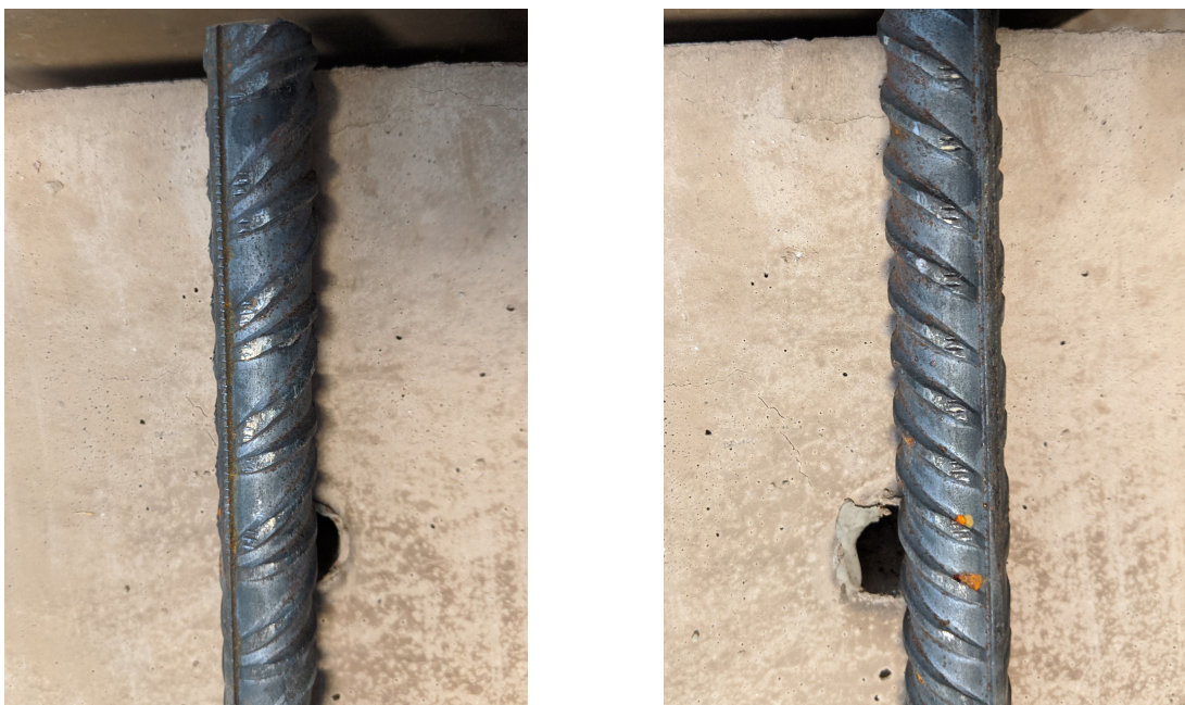
Fig. 3.1.3. Standard reinforcement bar with Ø20mm used in bond strength test.
