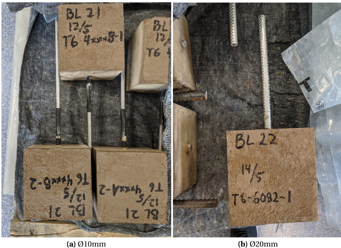
Fig. 3.7.1. Aluminium rebars cast in concrete.
