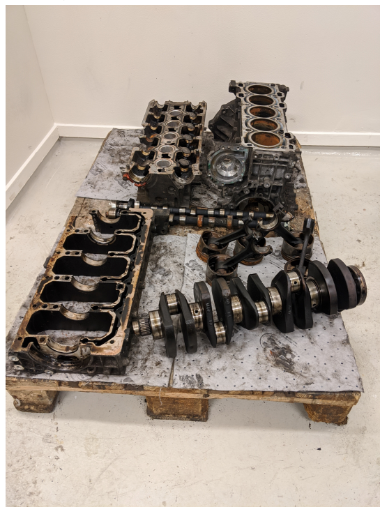
Fig. A.0.3. Disassembled engine. The engine block can be seen in the top right corner.
