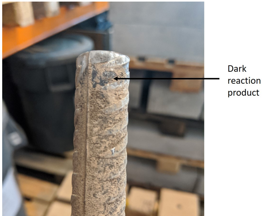
Fig. 4.4.8. T6-6082 reinforcement bar after bond strength test. A dark reaction product can be seen under the concrete residue.
