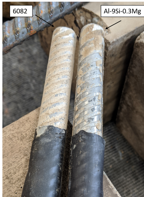
Fig. 5.3.1. Aluminium reinforcement after bond strength test. 6082 is covered in more concrete residue than Al-9Si-0.3Mg.
