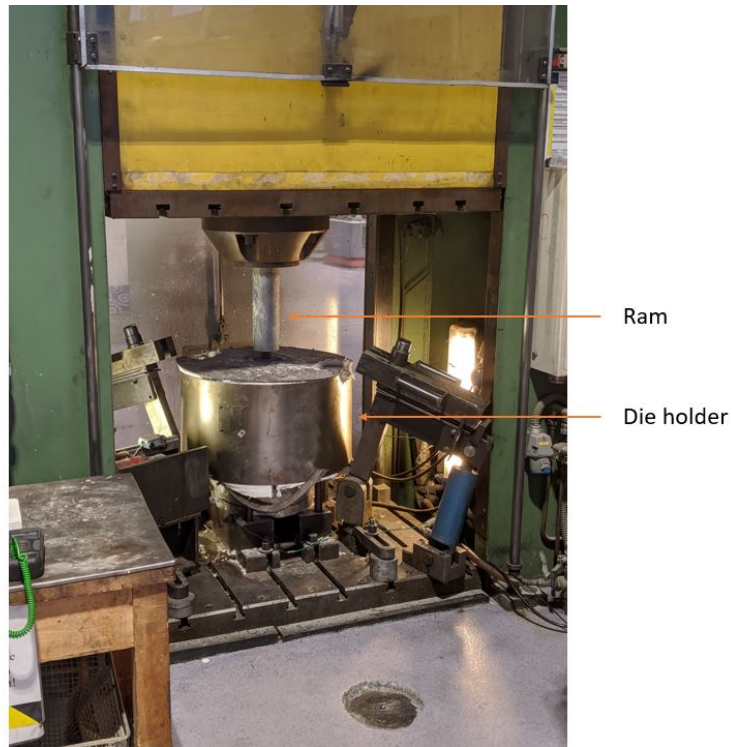
(a) Extruder at the first floor.
