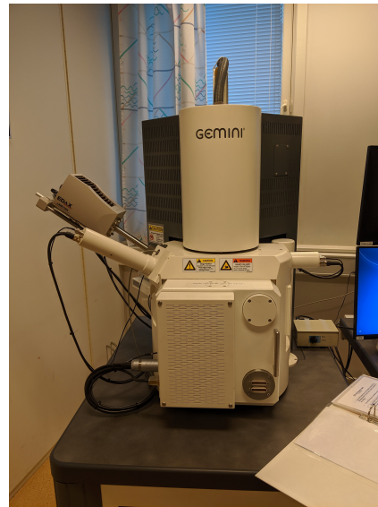
Fig. 3.2.3. Zeiss Supra 55VP used for SEM examinations. EDS attachment can be seen on the left, labeled as "EDAX".
