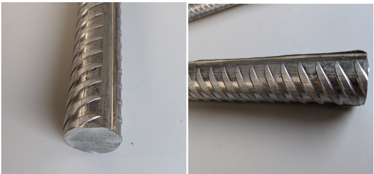
Fig. 4.2.2. Geometry of rolled \text{\O}20\text{mm} profiles.
