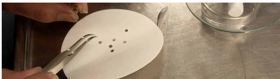
Figure 3.6: TEM samples after grinding and polishing. The samples were cut from the polished steel plate into samples with a diameter of 3 mm.
