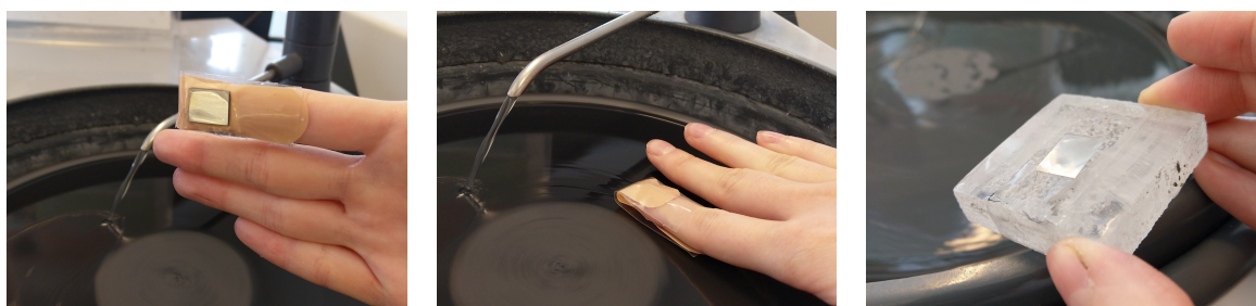
Figure 3.4: The images show the manual polishing with SiC foil paper of the TEM samples.
