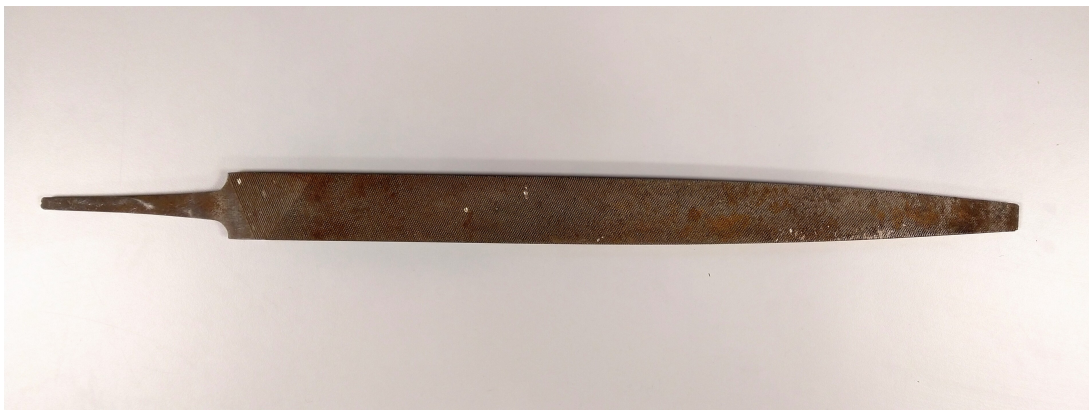
Figure 3.1: The steel as delivered, Alloy 1: 103Cr3/103C3. Full length about 50 cm.
